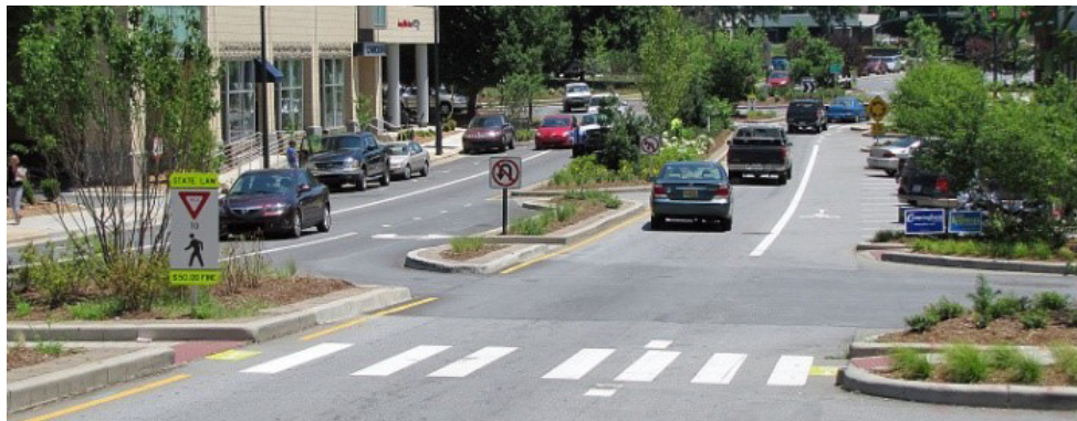
Curb extensions and medians make crossing four-lane streets safer and more manageable. (Credit: Dan Burden)
