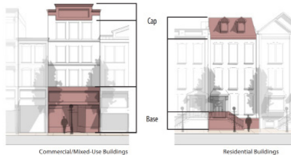
Figure 1.32: Building Base, Middle and Cap, Davidson, NC
