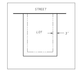
PUBLIC STORMWATER DRAINAGE EASEMENTS (SEE NOTE 2) NOT TO SCALE
