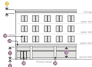
Figure 3903(g)-E. Storefront Building Facade
