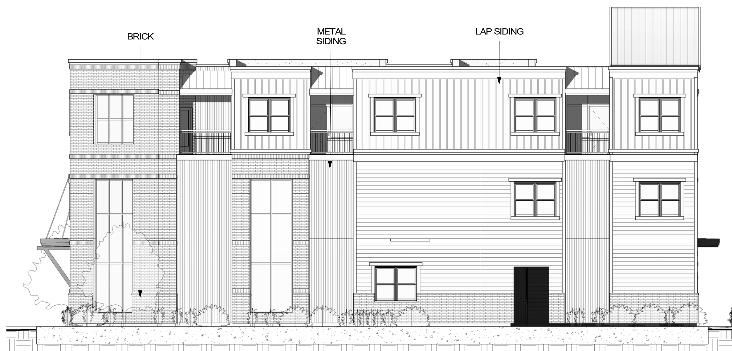
4 WEST BUILDING ELEVATION A3.1 1/8" = 1'-0"
