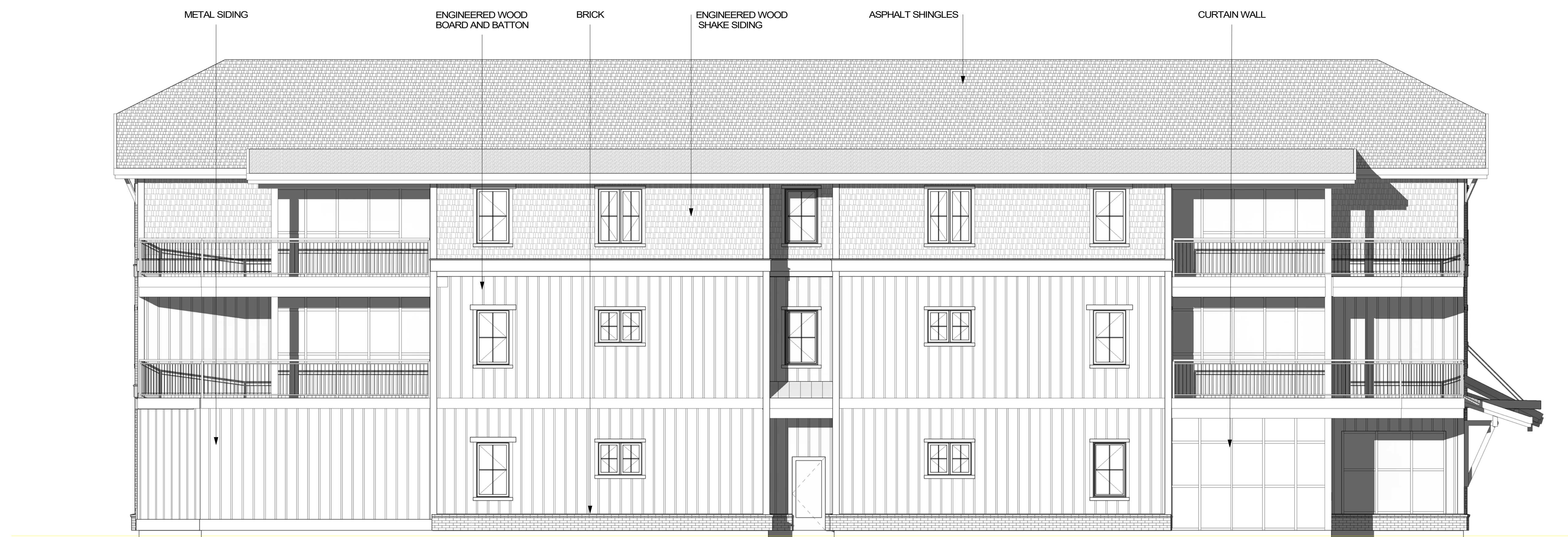
SOUTH BUILDING ELEVATION
