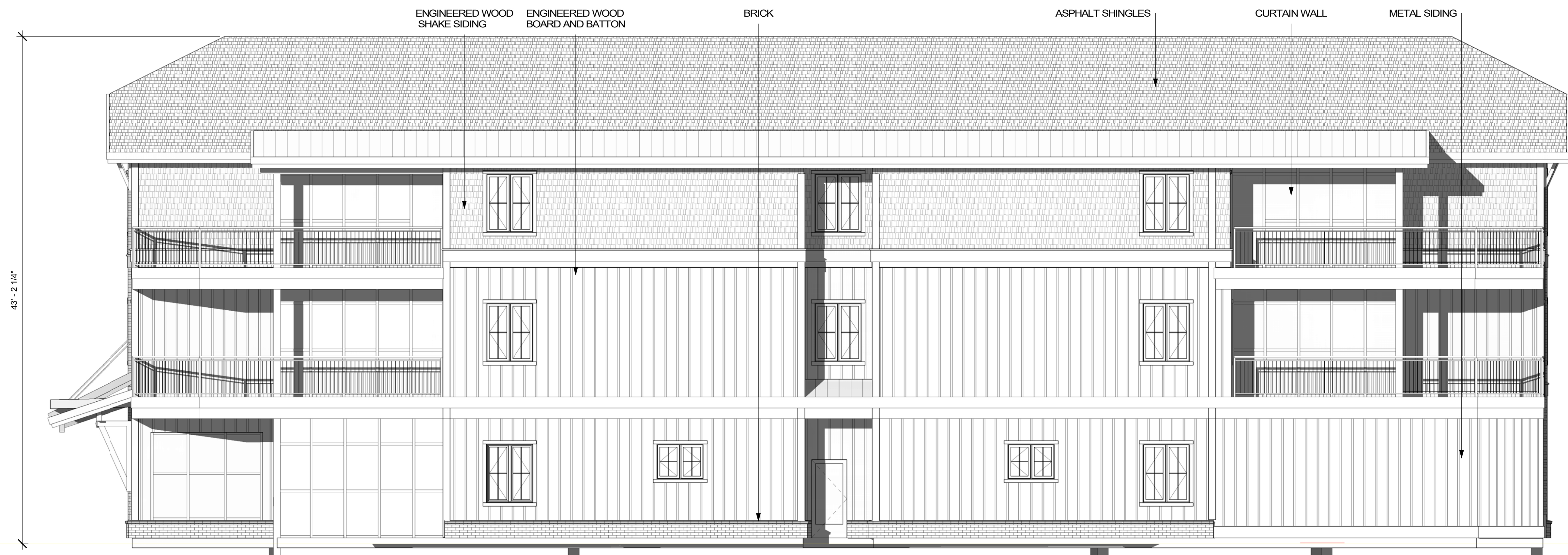
2 NORTH BUILDING ELEVATION A3.1 3/16" = 1'-0"
