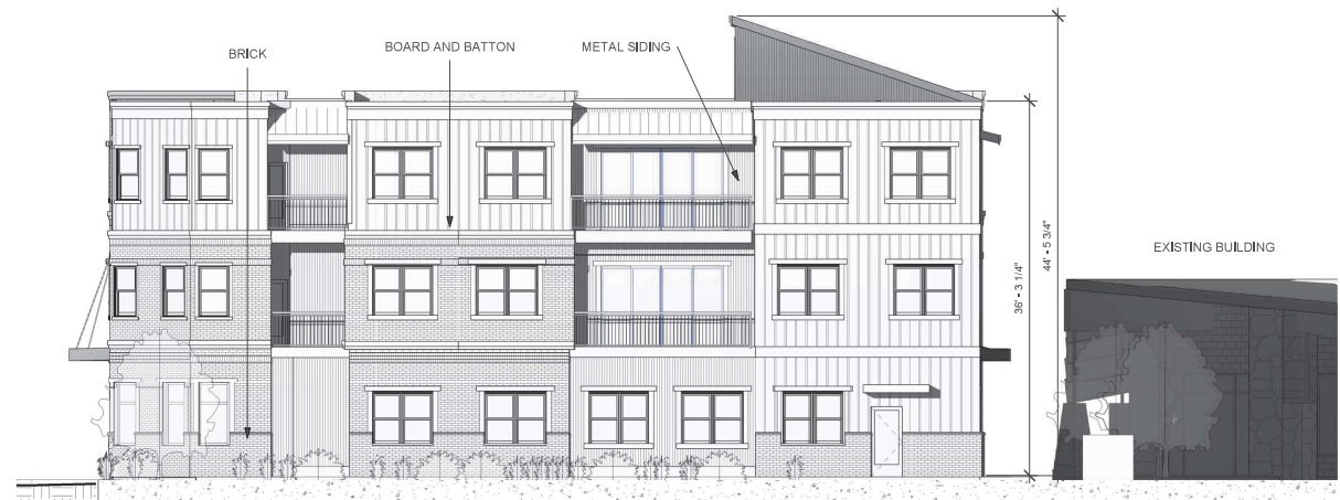
4 WEST BUILDING ELEVATION A3.1 1/8" = 1'-0"
