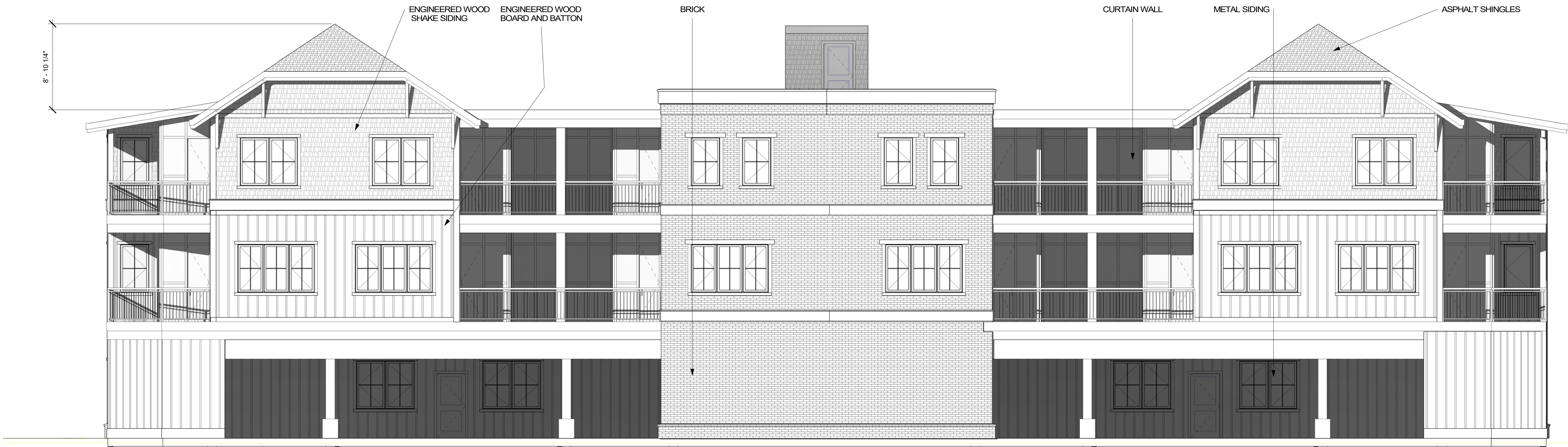
2 WEST BUILDING ELEVATION A3.2 3/16" = 1'-0"
