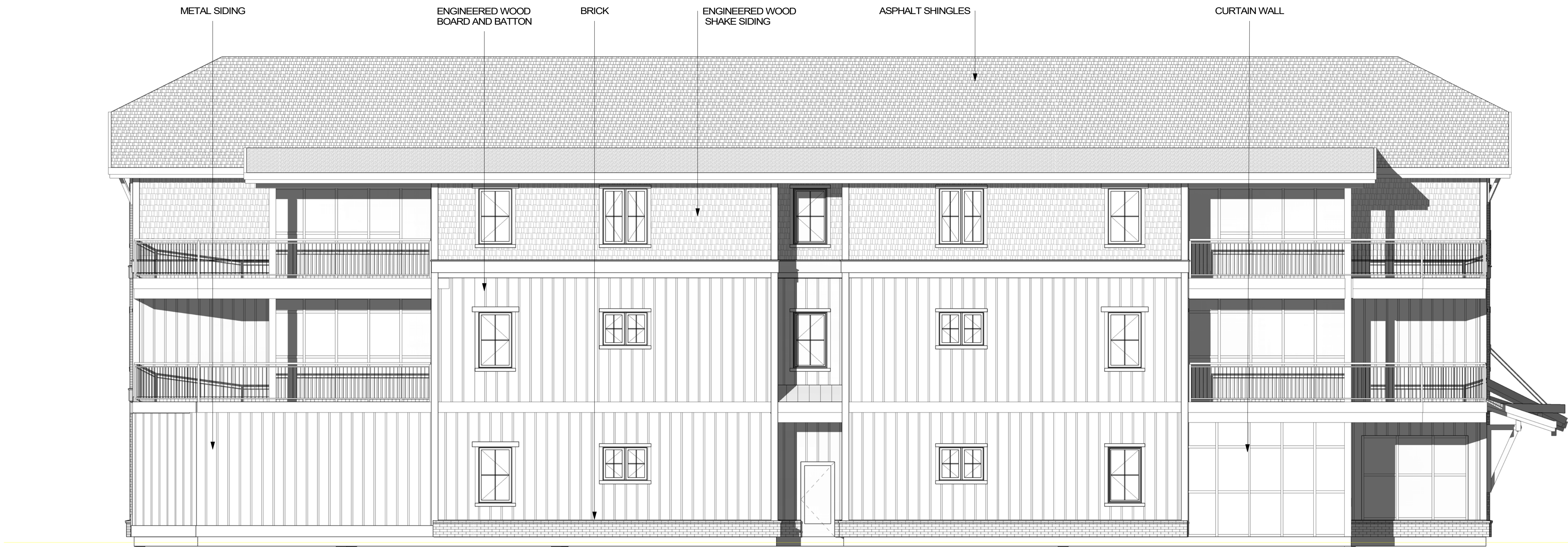
1 SOUTH BUILDING ELEVATION A3.2 3/16" = 1'-0"
