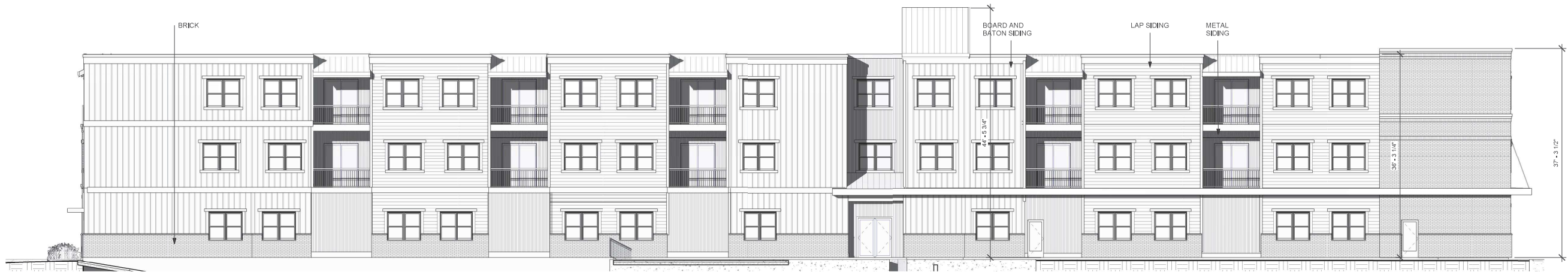
3 SOUTH BUILDING ELEVATION 1/8" = 1'-0"
