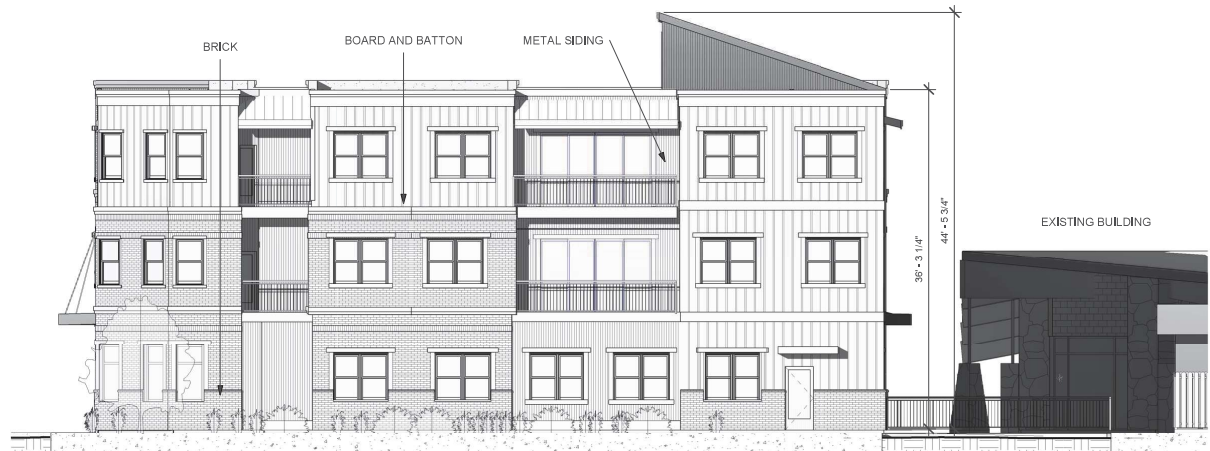
4 WEST BUILDING ELEVATION 1/8" = 1'-0"
