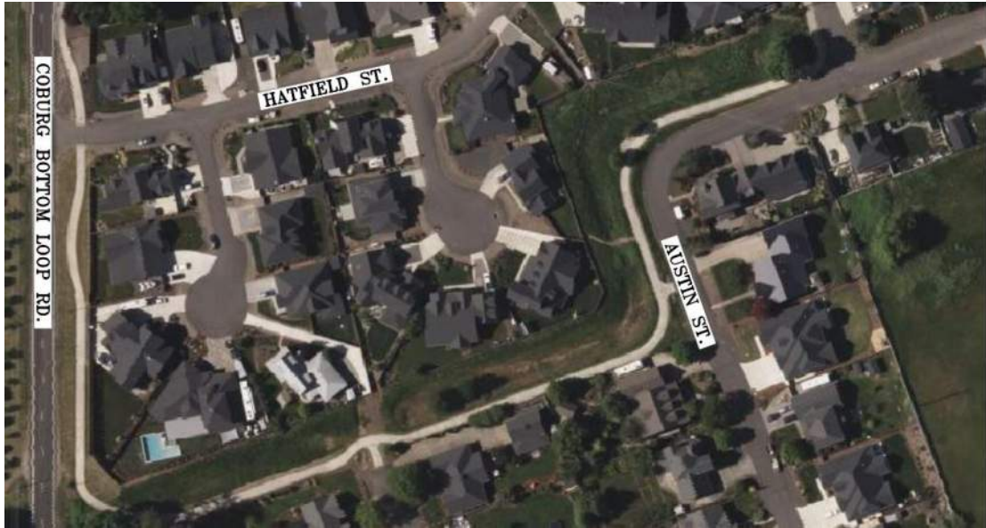
Figure 1: Detention swales in NE of Coburg, with overflow draining into tributary to Muddy Creek
