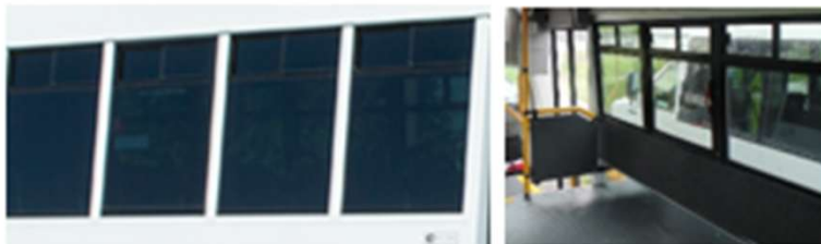
T-slide and carpet/panel below windows
