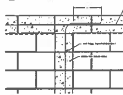
34.3 BOND BEAM VERTICAL BAR TERMINATION DETAIL SCALE: 1" = 1'-0"
