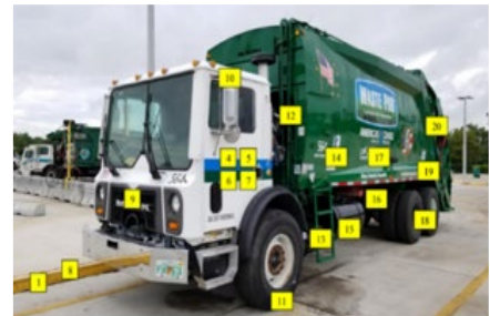
Each numbered yellow box represents an inspection point. Our focus on safety means fewer maintenance issues, lower environmental impact, and fewer service delays for Pensacola.
