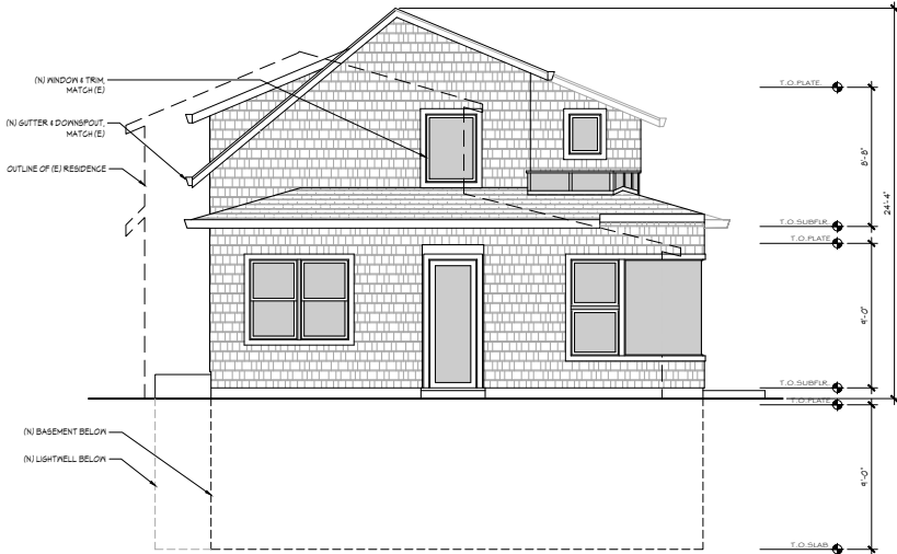
2 NORTH ELEVATION SCALE: 1/4" = 1'-0"
