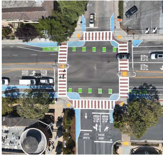
Example road diet and traffic calming features implemented at the existing all-way stop at Bay/Hill (Capitola)
