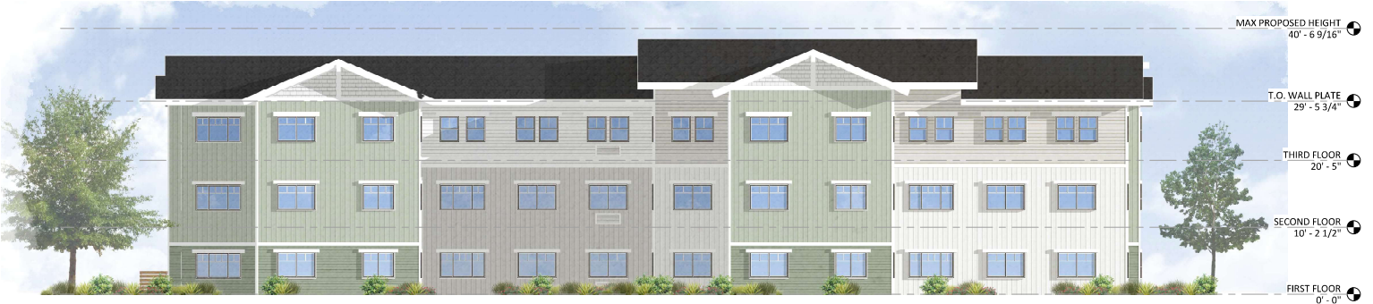
BUILDING C - SOUTH ELEVATION | 1/8" = 1'-0" | 1
