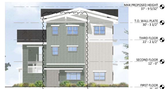
BUILDING B - EAST ELEVATION | 1/8" = 1'-0" | 2
