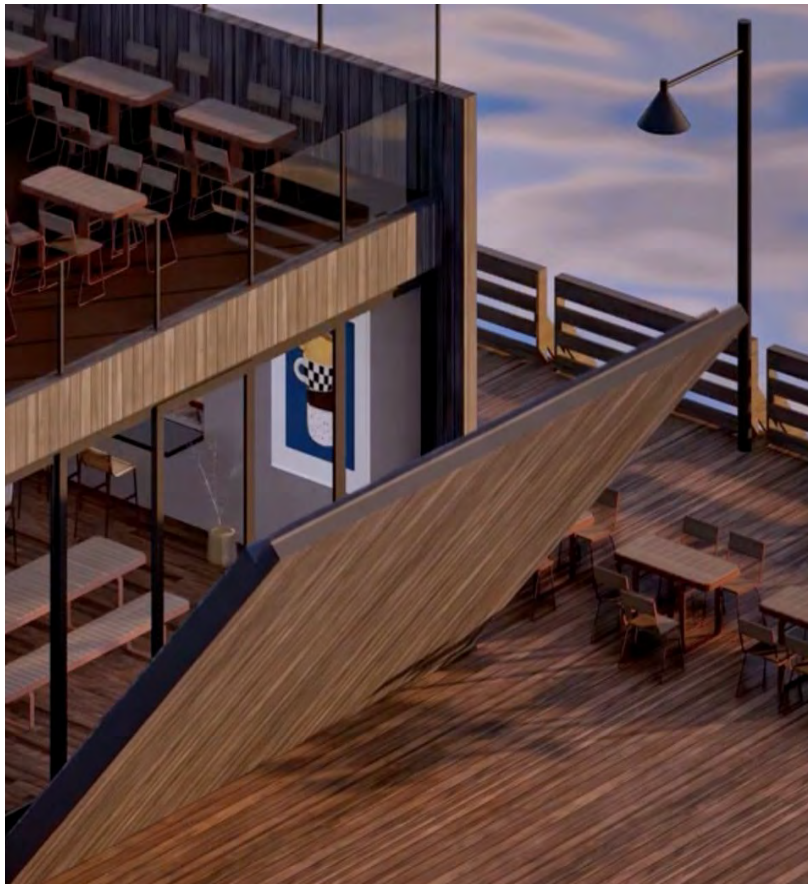
'FLIP-UP DECK' FOR BAD WEATHER, WIND & PROJECTILE DEFENSE
