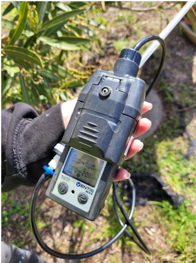
Figure 8. Ventis MX-4 Handheld Multi-Gas Detector
