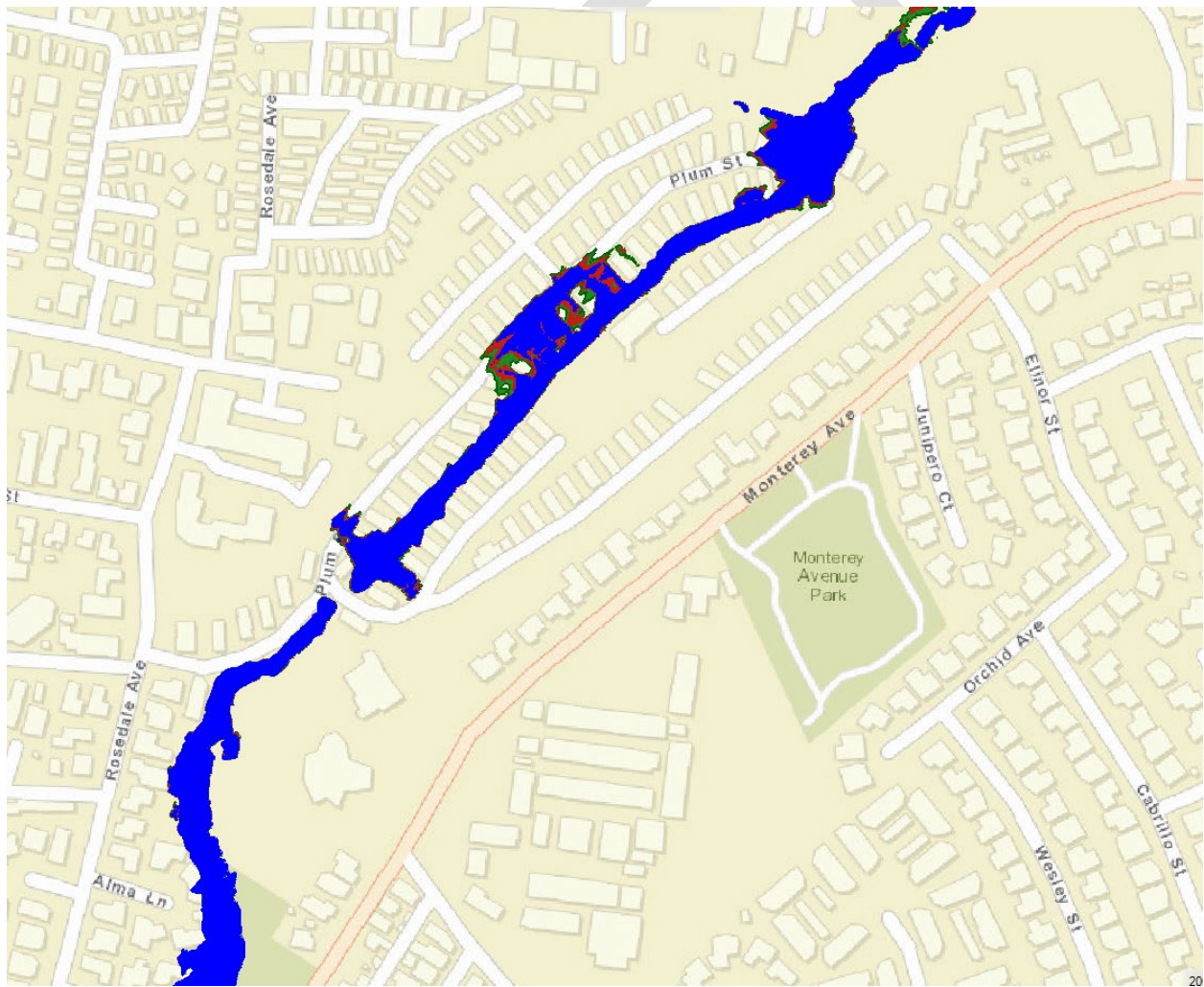
Figure 5-7: Noble 100-yr HEC-RAS (with Existing Culverts) Climate Change Model Inundation, Including Existing Condition (Blue), with 12% Increase in Runoff (Red), and with 25% Increase in Runoff (Green)
