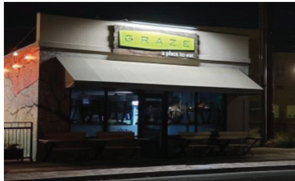
Figure 104. Example of facade fixture where a linear wash of light illuminates a sign in Walla Walla, WA [Photo credit: Seanette Corkill]
