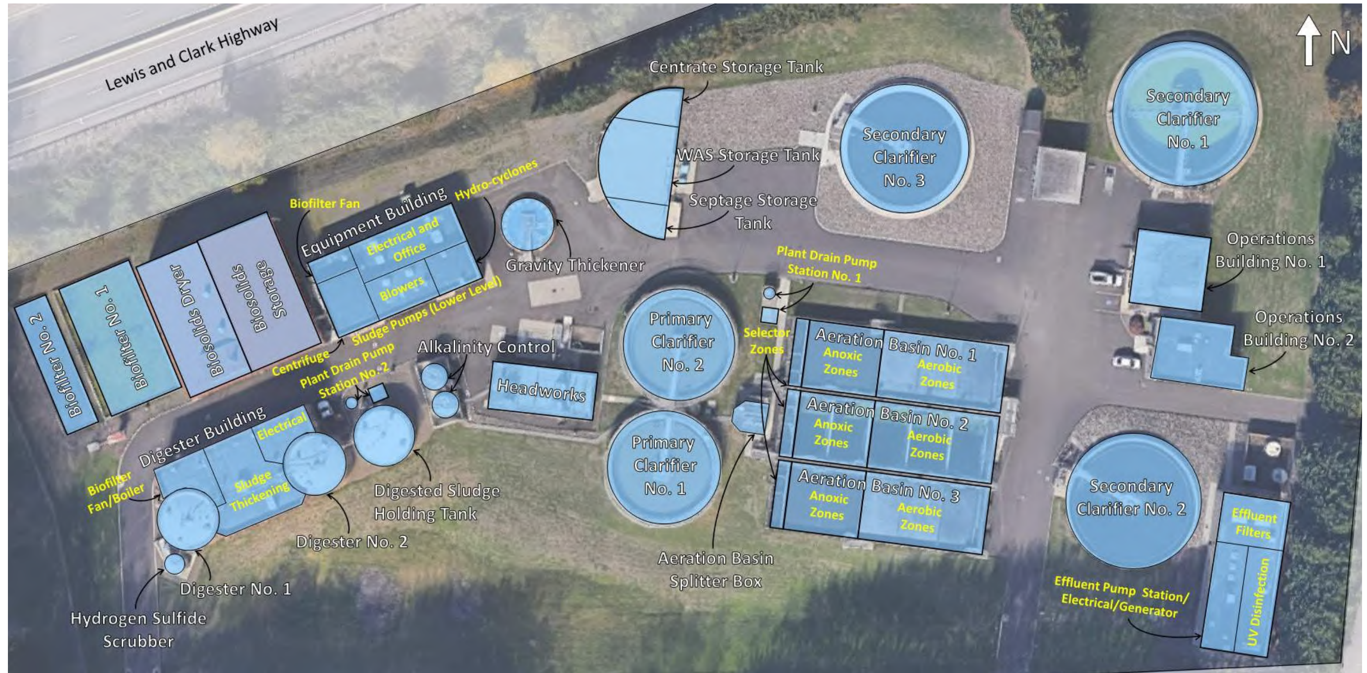
Figure 4.5 WWTf Aerial Image with Site Plan
