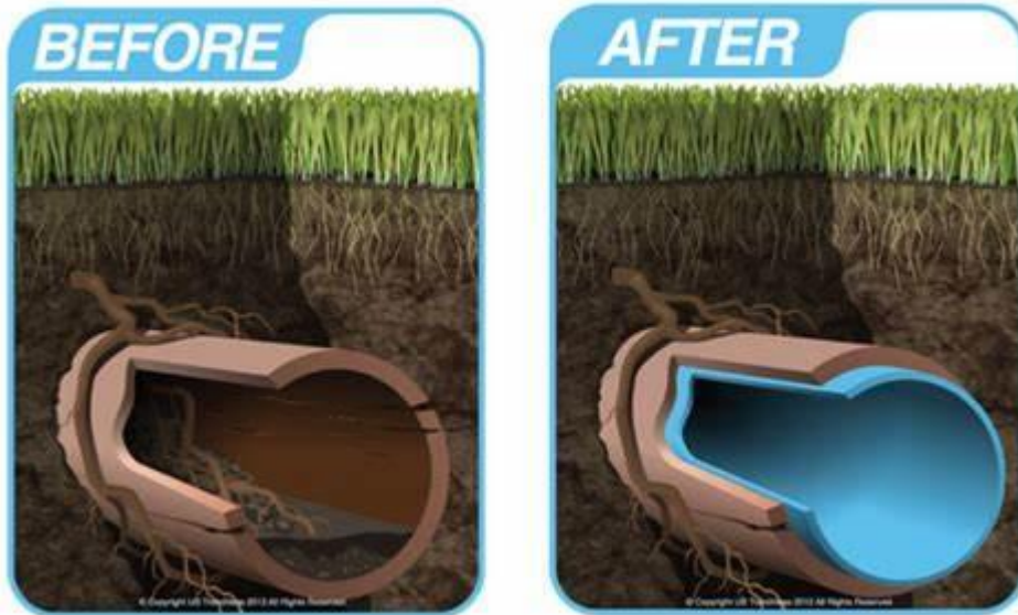
Figure 2. Illustration of before and after CIPP
