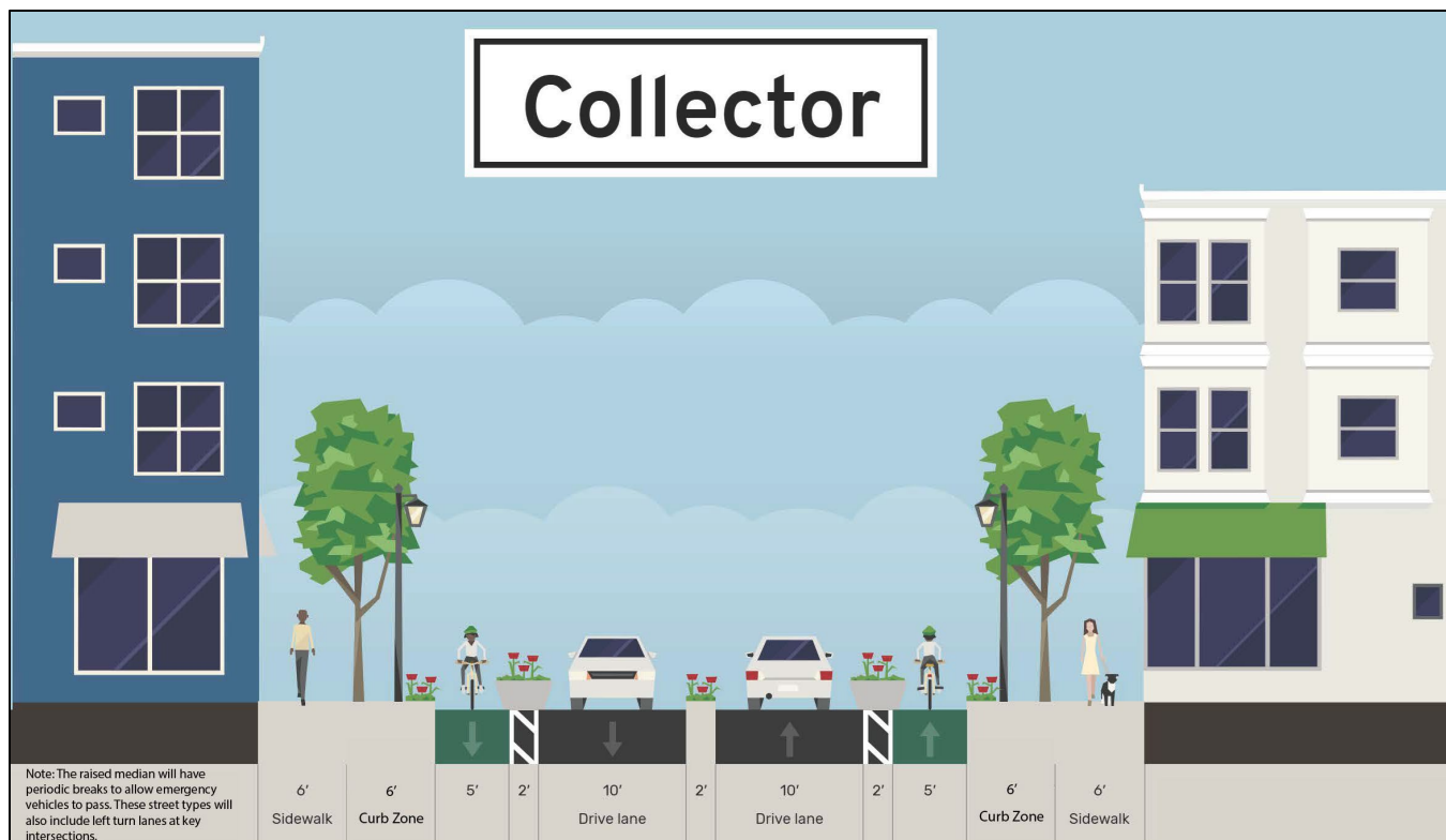
Figure 16. Collector Road Cross Section
