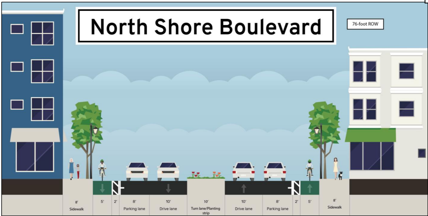
Figure 14. North Shore Boulevard Cross Section
