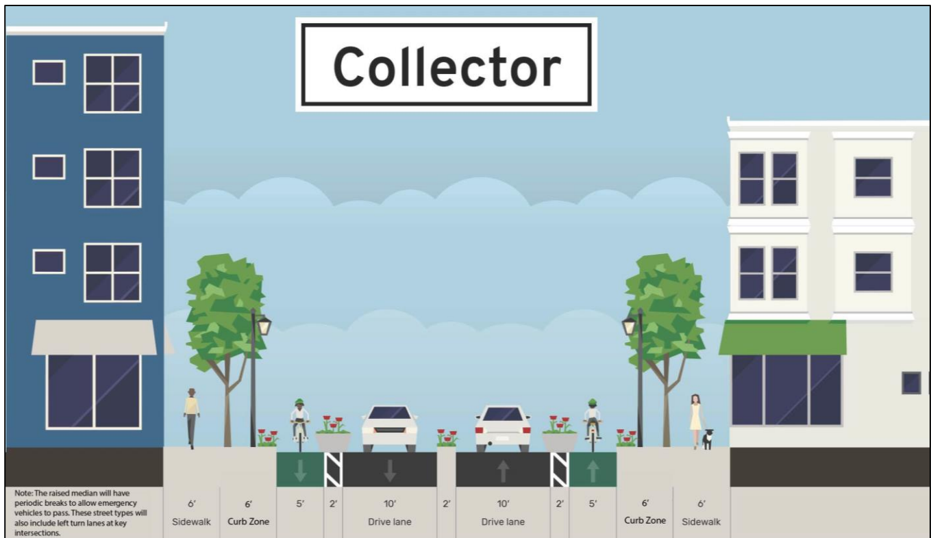
Figure 16. Collector Road Cross Section
