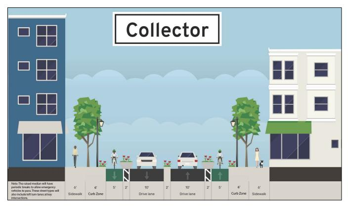
Figure 16. Collector Road - Conceptual Cross Section
