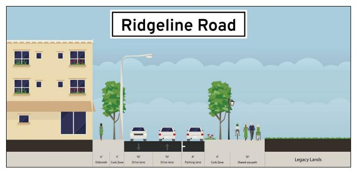
Figure 15. Ridgeline Road - Conceptual Cross Section
