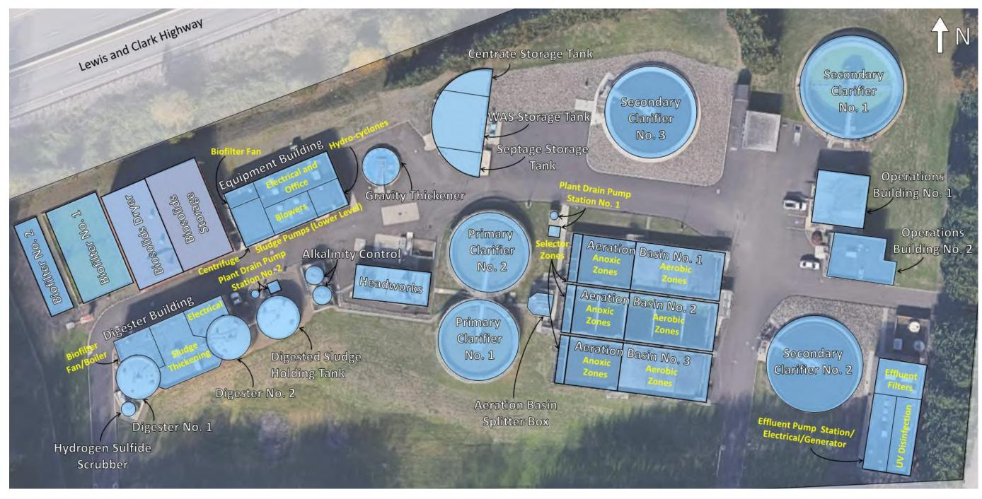
Figure 4.5 WWTF Aerial Image with Site Plan
