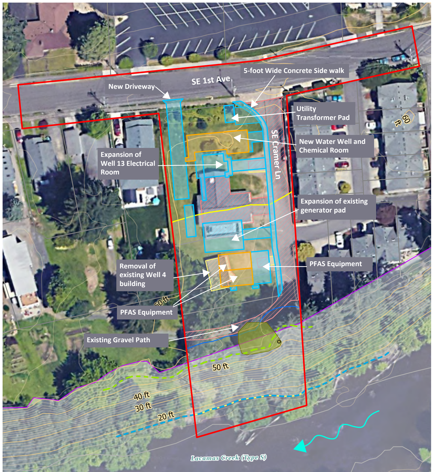
Figure 3. Proposed Conditions Camas Well 13 PFAS Treatment Design
