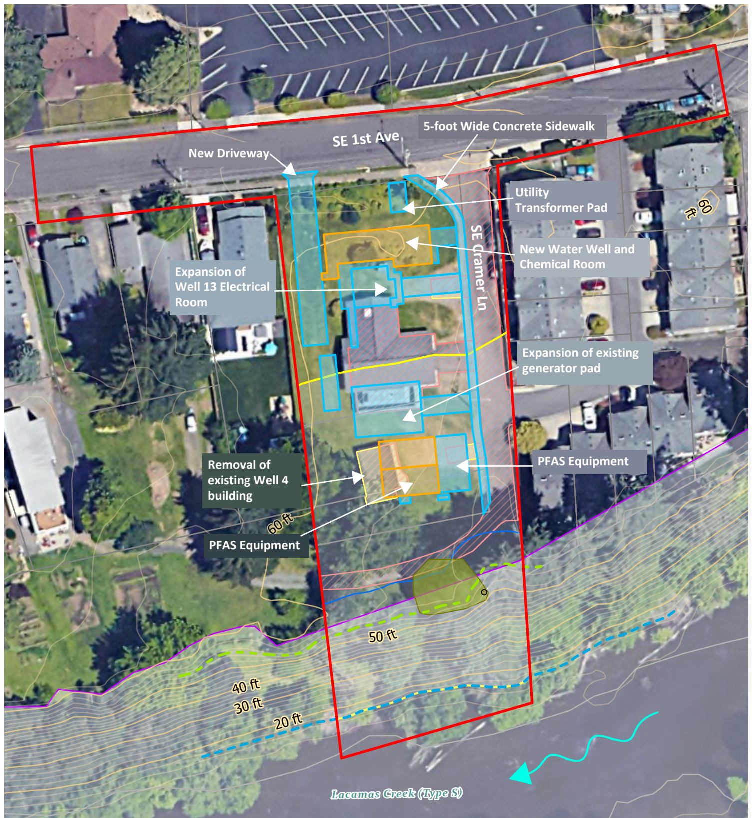
Figure 3. Proposed Conditions Camas Well 13 PFAS Treatment Design
