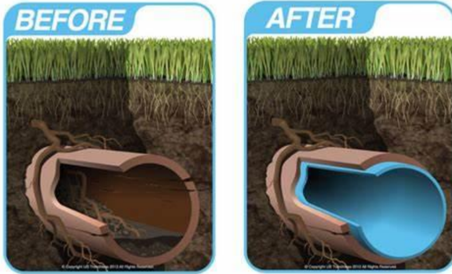
Figure 2. Illustration of before and after CIPP
