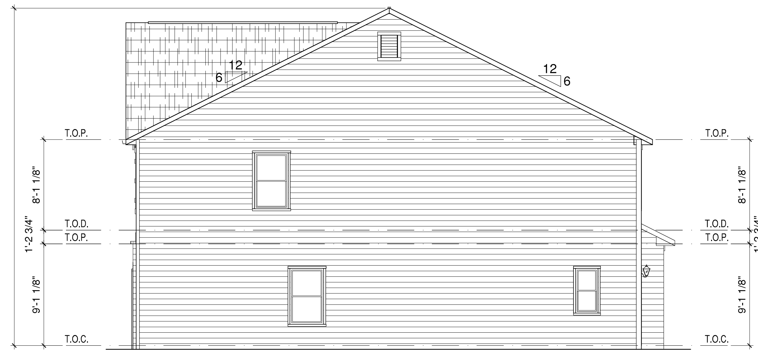
2 BUILDING B - END ELEVATION - "STYLE A" SCALE: 3/16"=1'-0"
