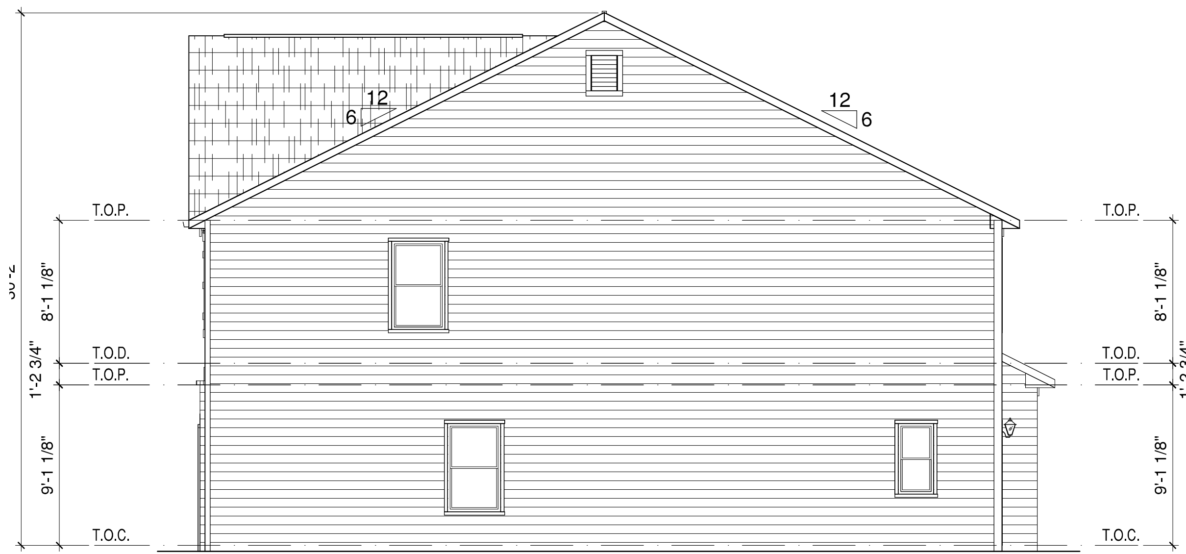
2 BUILDING B - END ELEVATION - "STYLE B" SCALE: 3/16"=1'-0"
