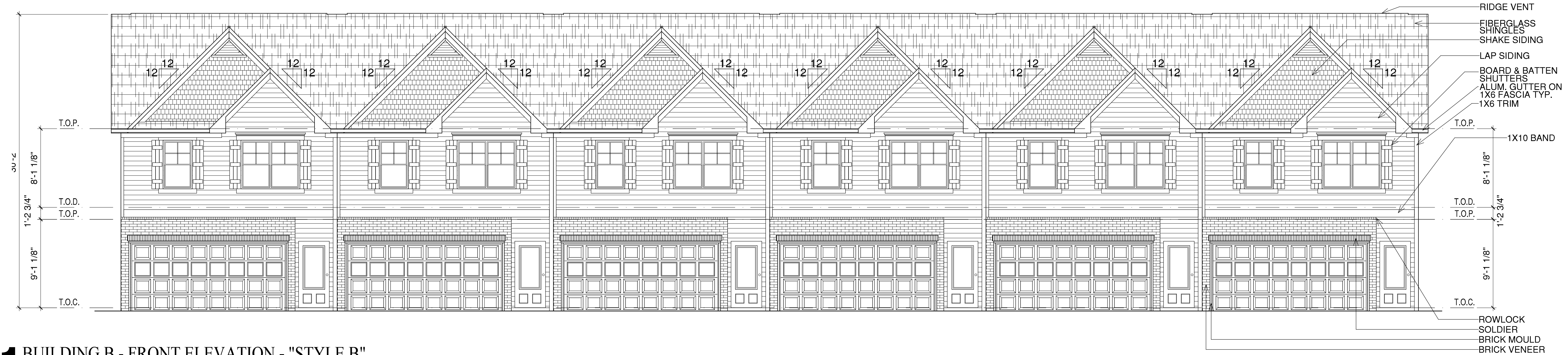
1 BUILDING B - FRONT ELEVATION - "STYLE B" SCALE: 3/16"=1'-0"
