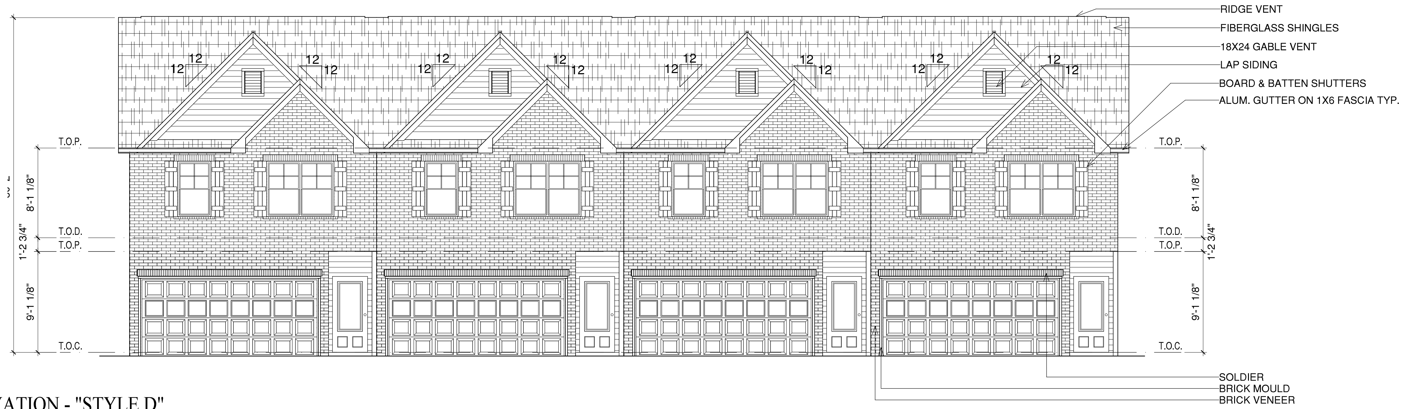
1 BUILDING A - FRONT ELEVATION - "STYLE D" SCALE: 1/8"=1'-0"
