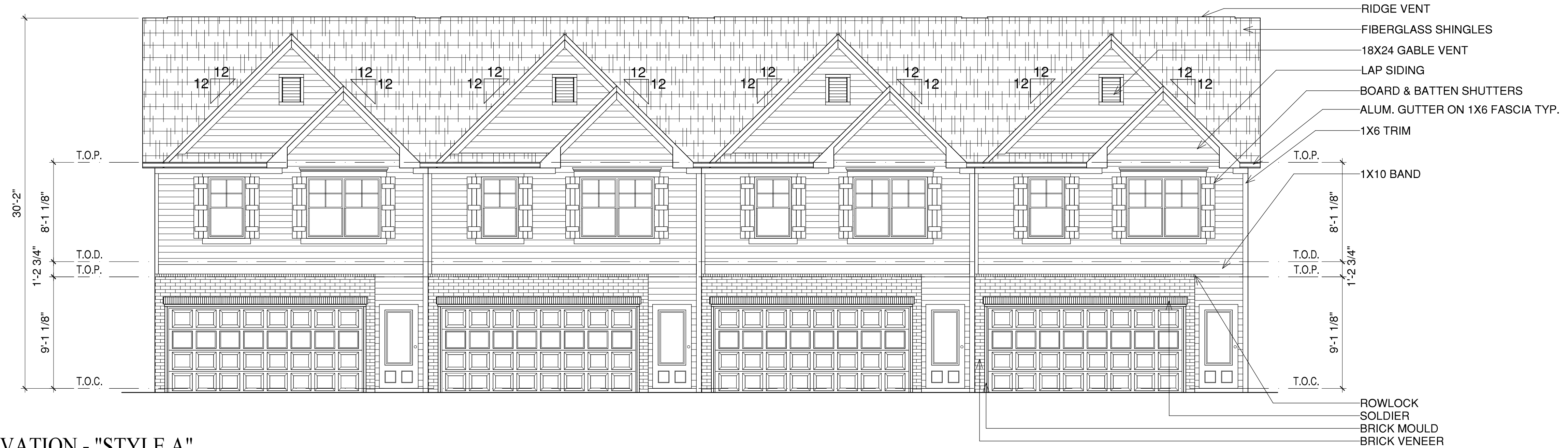
1 BUILDING A - FRONT ELEVATION - "STYLE A" SCALE: 3/16"=1'-0"
