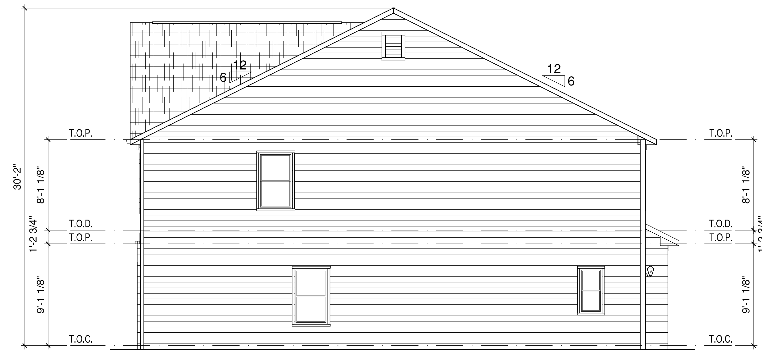
2 BUILDING A - END ELEVATION - "STYLE A" SCALE: 3/16"=1'-0"
