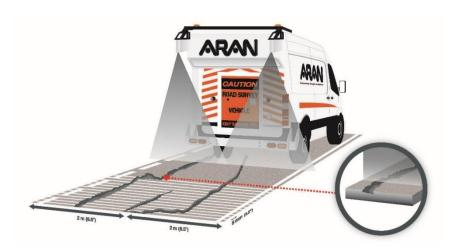
**Figure 5: Downward Scanning Capabilities**
