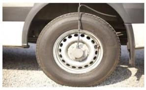
Figure 3: Distance Measuring Instrument (DMI)
