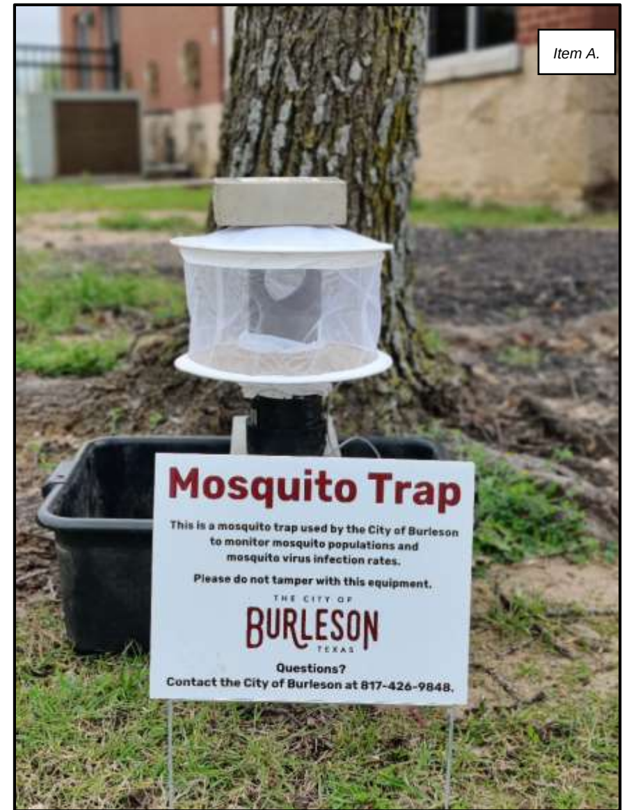
Gravid trap for collecting mosquitoes
