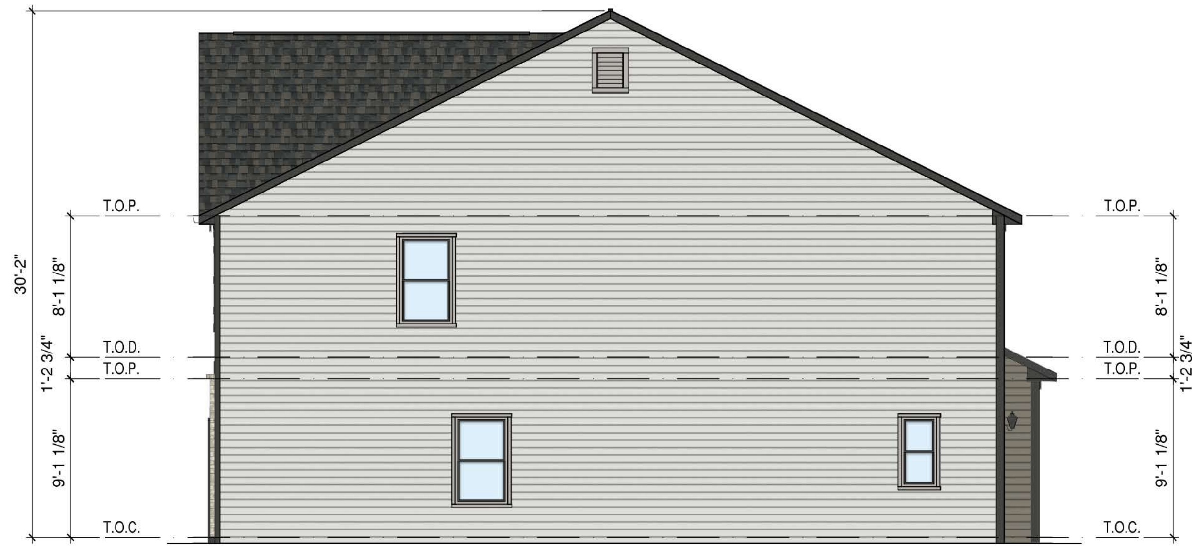
2 BUILDING A - END ELEVATION - "STYLE B" SCALE: 3/16"=1'-0"
