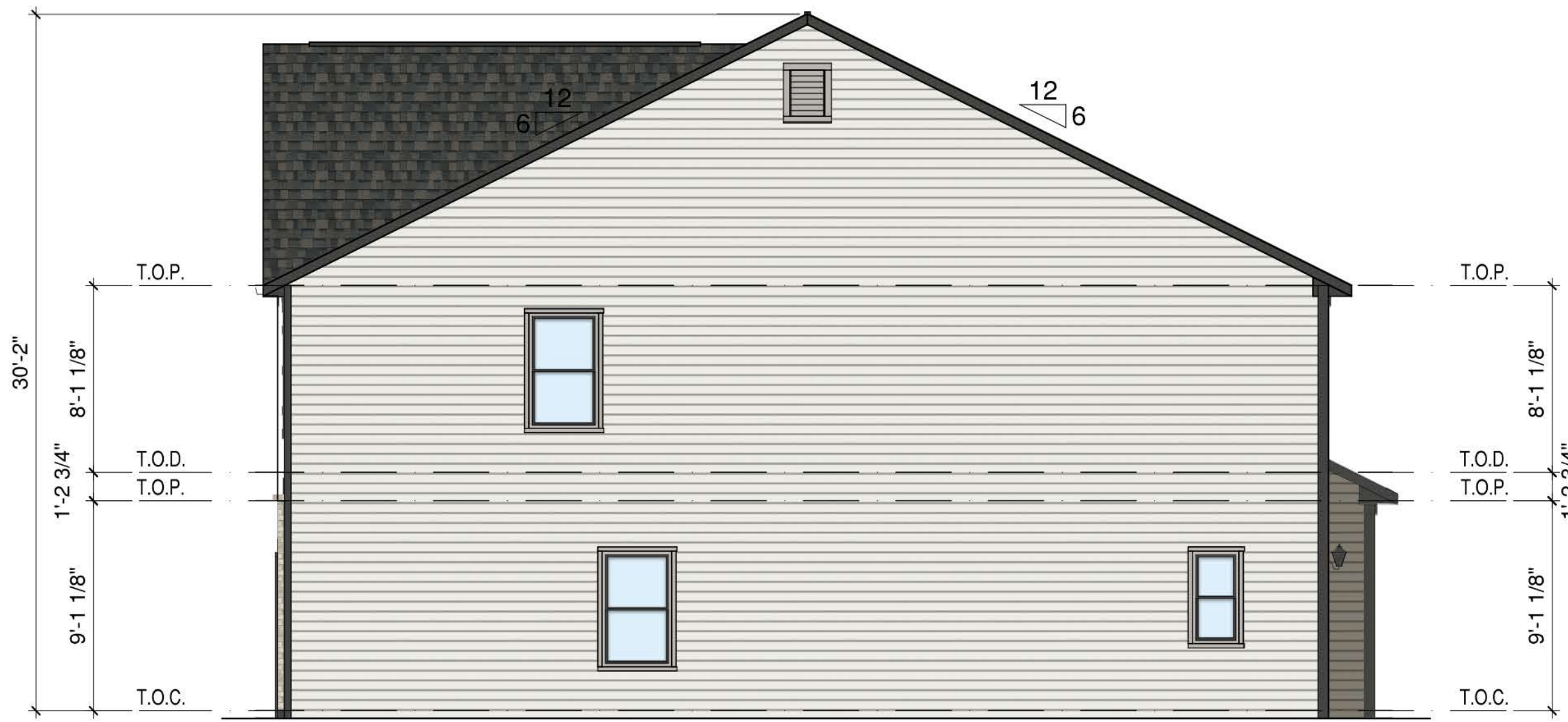
2 BUILDING A - END ELEVATION - "STYLE D" SCALE: 1/8"=1'-0"
