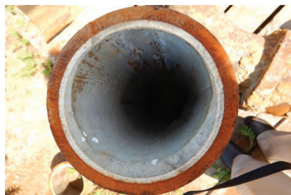
Old cast iron pipe with new cement lining.
