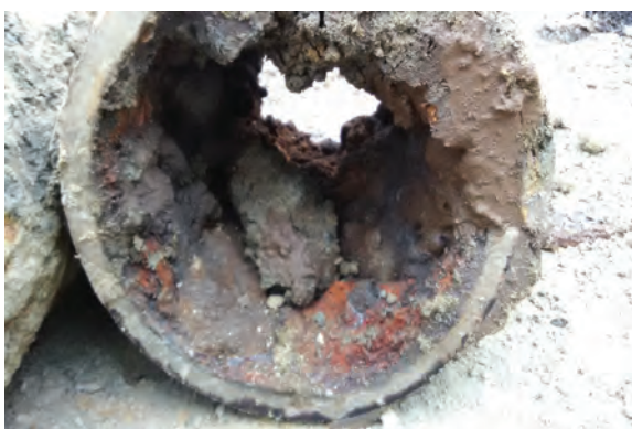
Old cast iron pipe before cleaning and lining.
