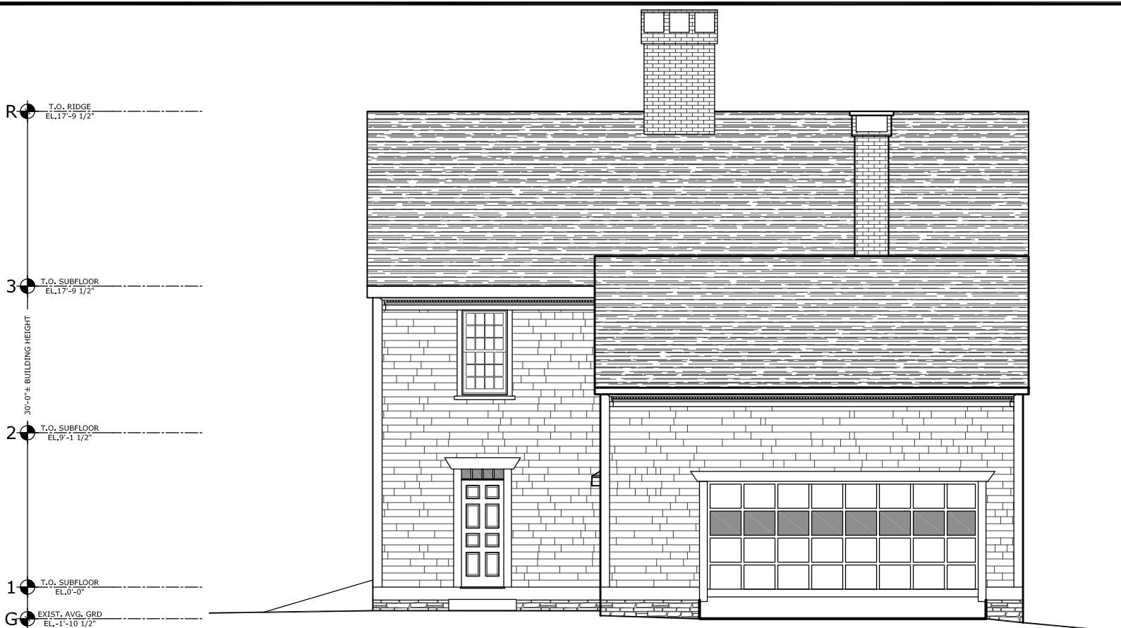
1 EXISTING EAST ELEVATION
