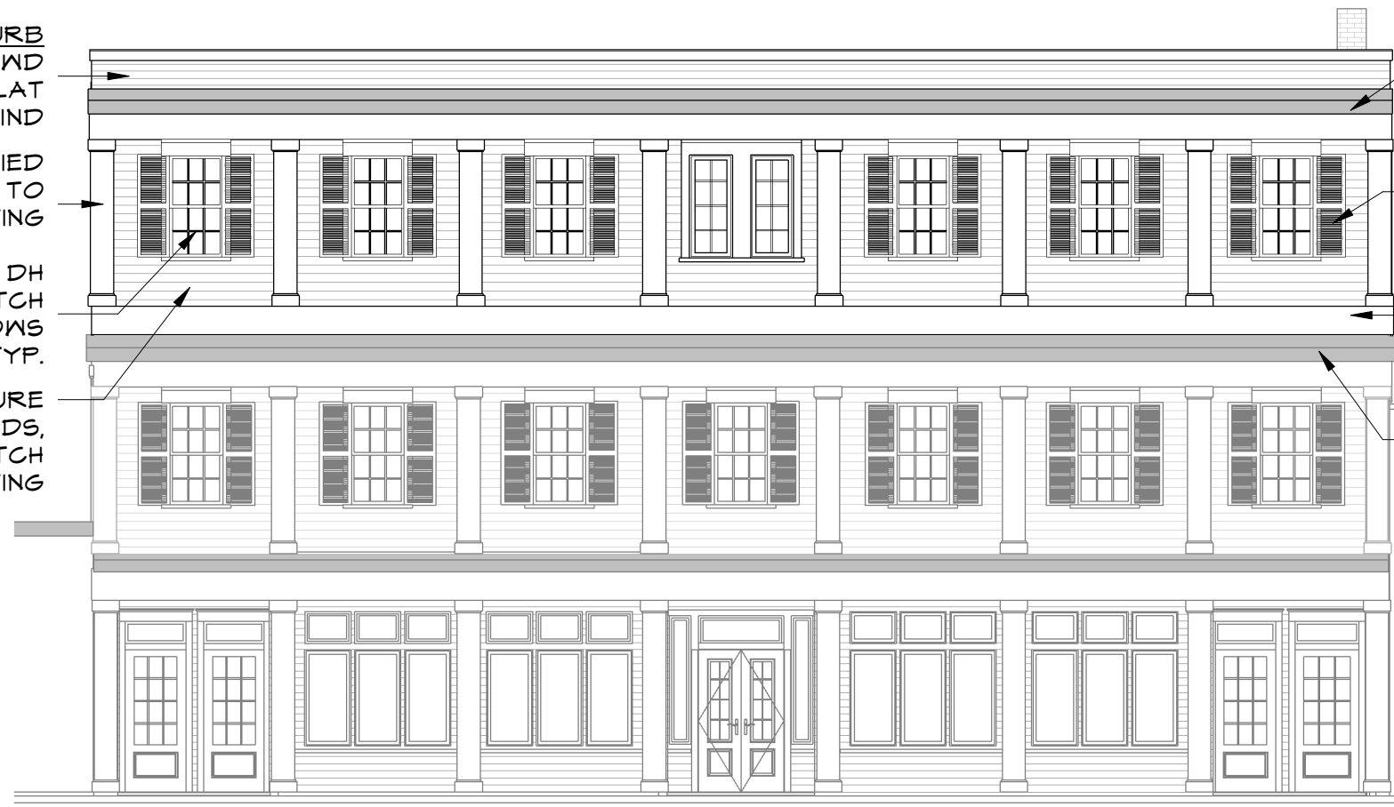
① NEW EAST ELEVATION HDC 1/8" = 1'-0"
