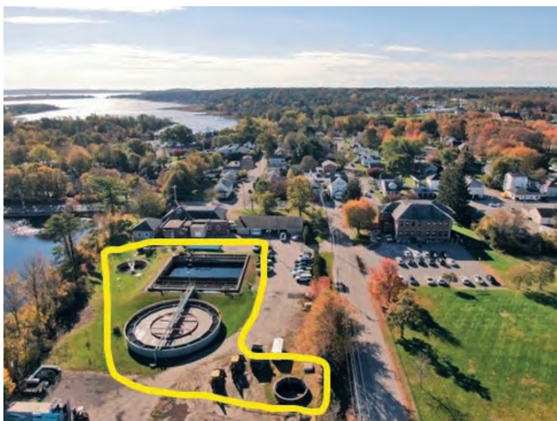
Phase I demolition of the obsolete treatment plant includes the exterior tank structures and piping.
