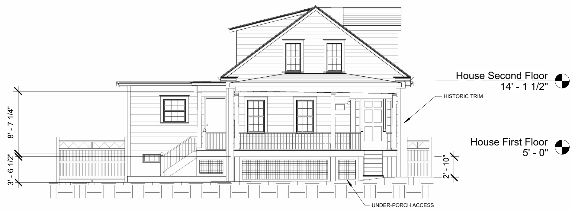
① Existing South Elevation 1/8" = 1'-0"
