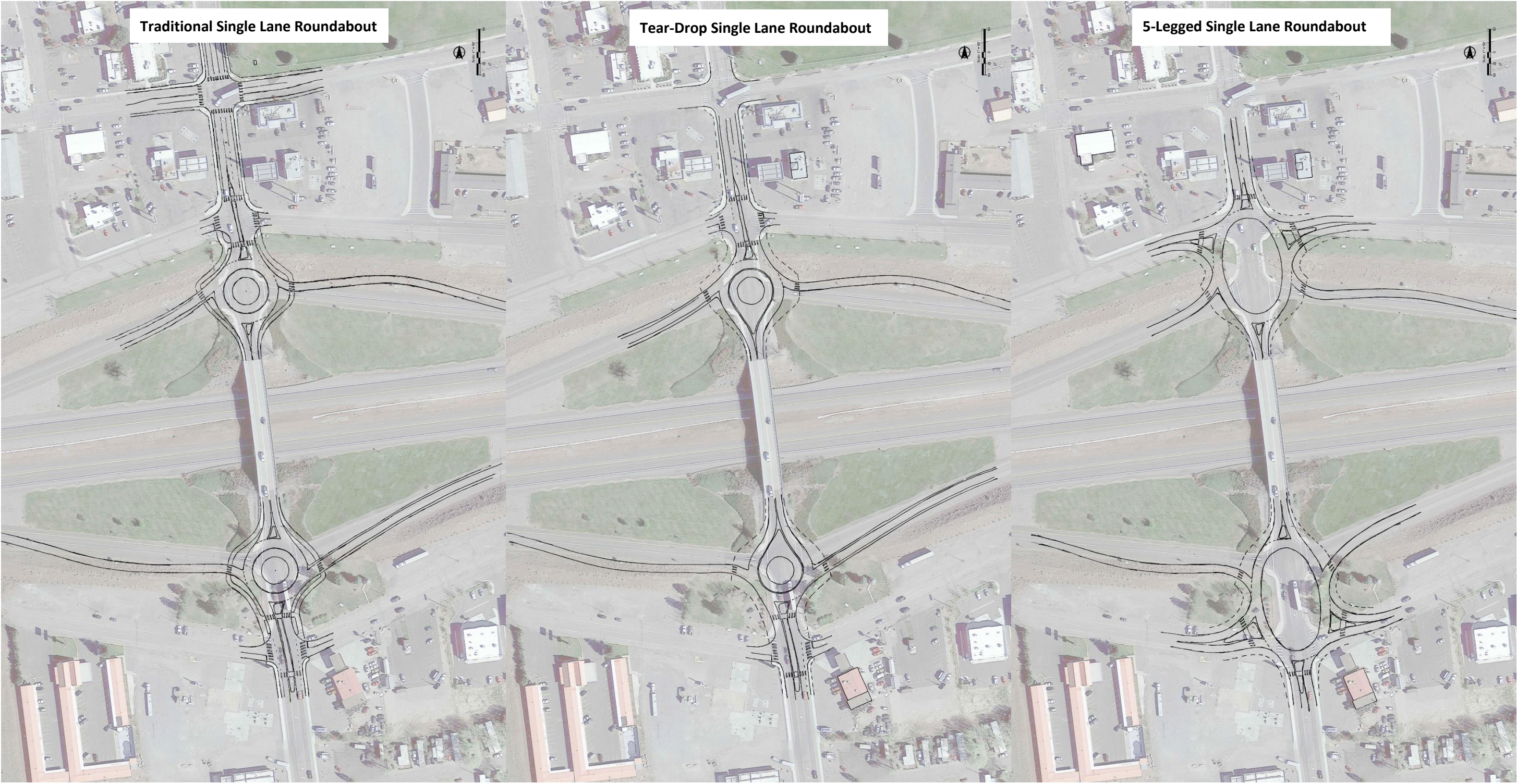
Figure 6 – Refined Sketch Level Layout of the I-84 EB and WB Ramp Terminals (for illustrative purposes only)
