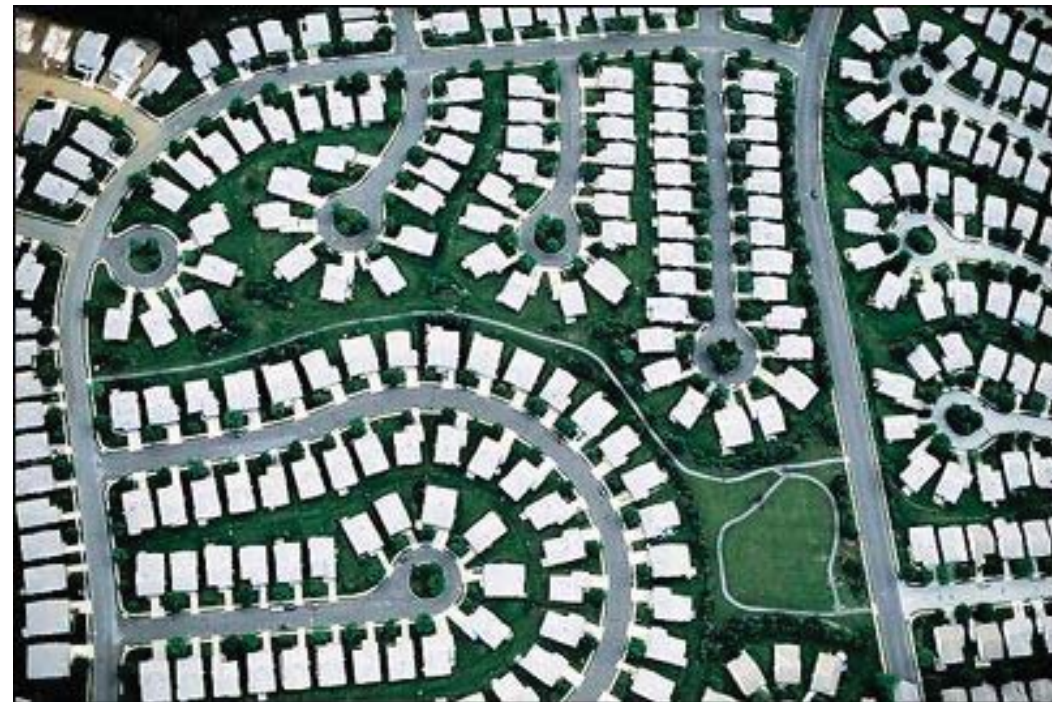
Figure 89: Bluffton's abundance of cul-de-sacs result in poor circulation and have negative traffic impacts.
