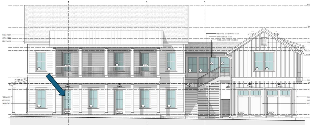
Fig 1. Door Replacement on West Elevation
