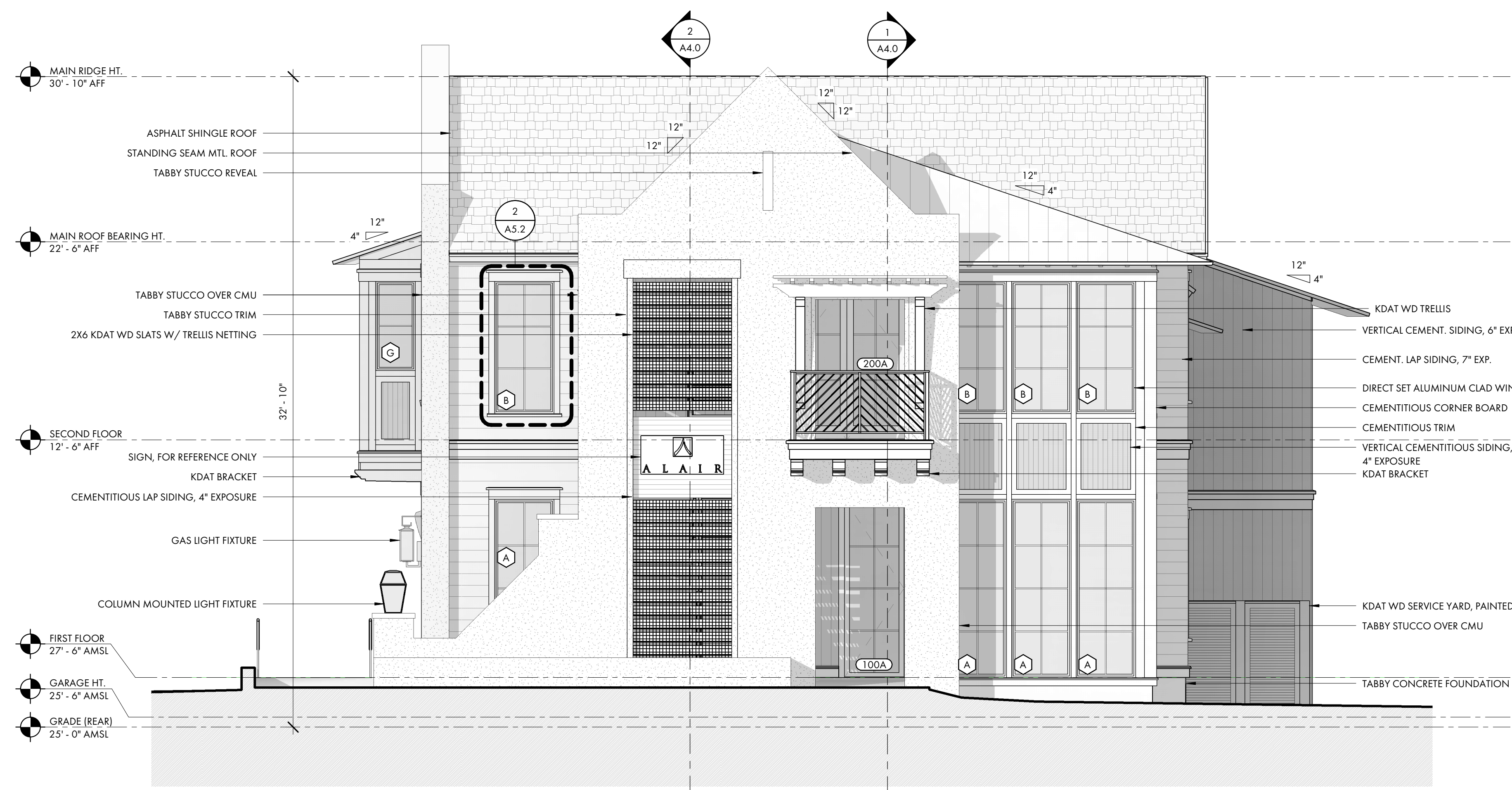
1 FRONT (NORTH) ELEVATION A3.0 1/4" = 1'-0"
