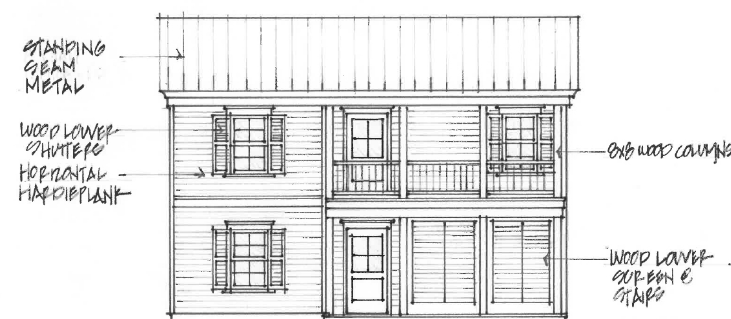
West Elevation \frac{1}{8}" = 1'-0"
