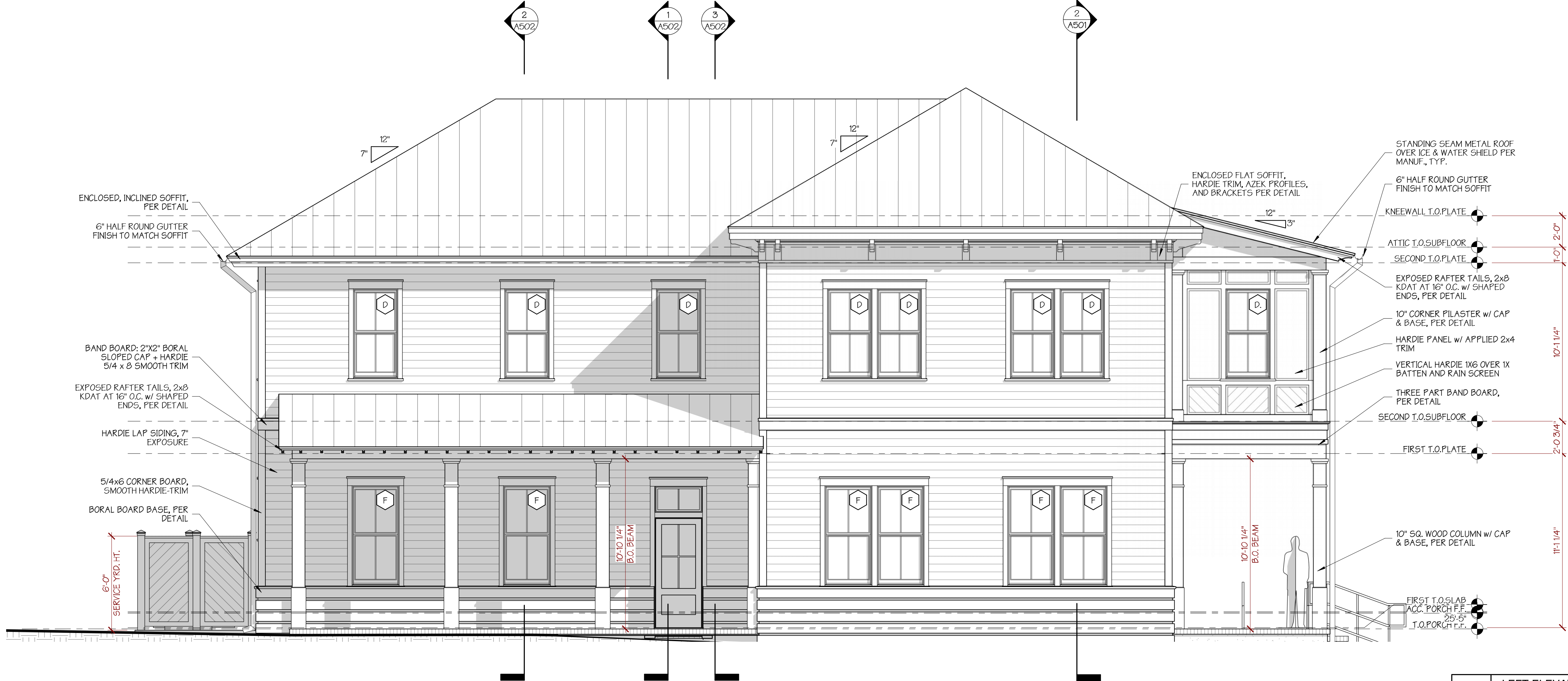
2 LEFT ELEVATION, PRIMARY 1/4" = 1'-0"
