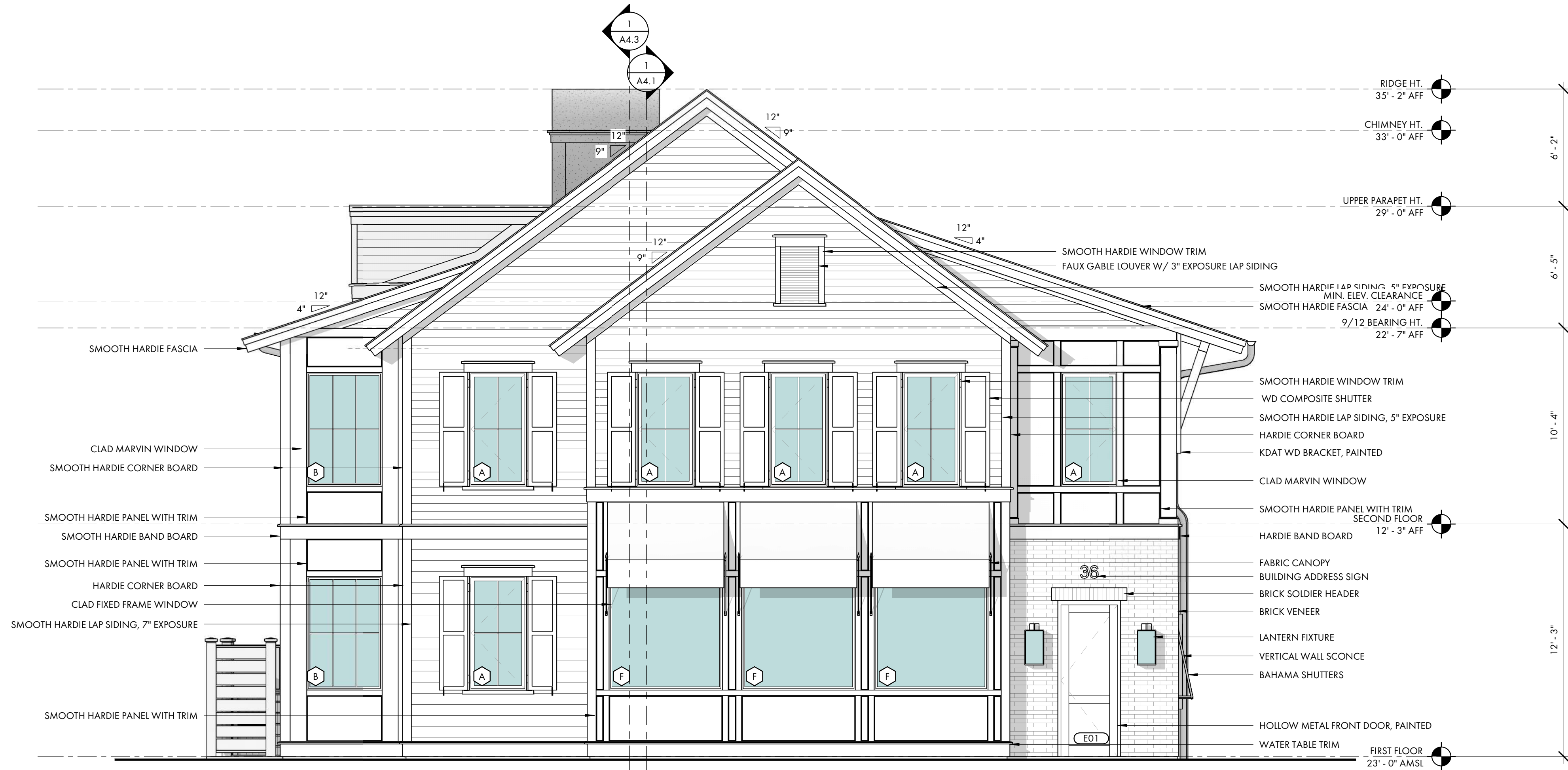
1 FRONT (BRUIN ROAD) ELEVATION A3.0 1/4" = 1'-0"
