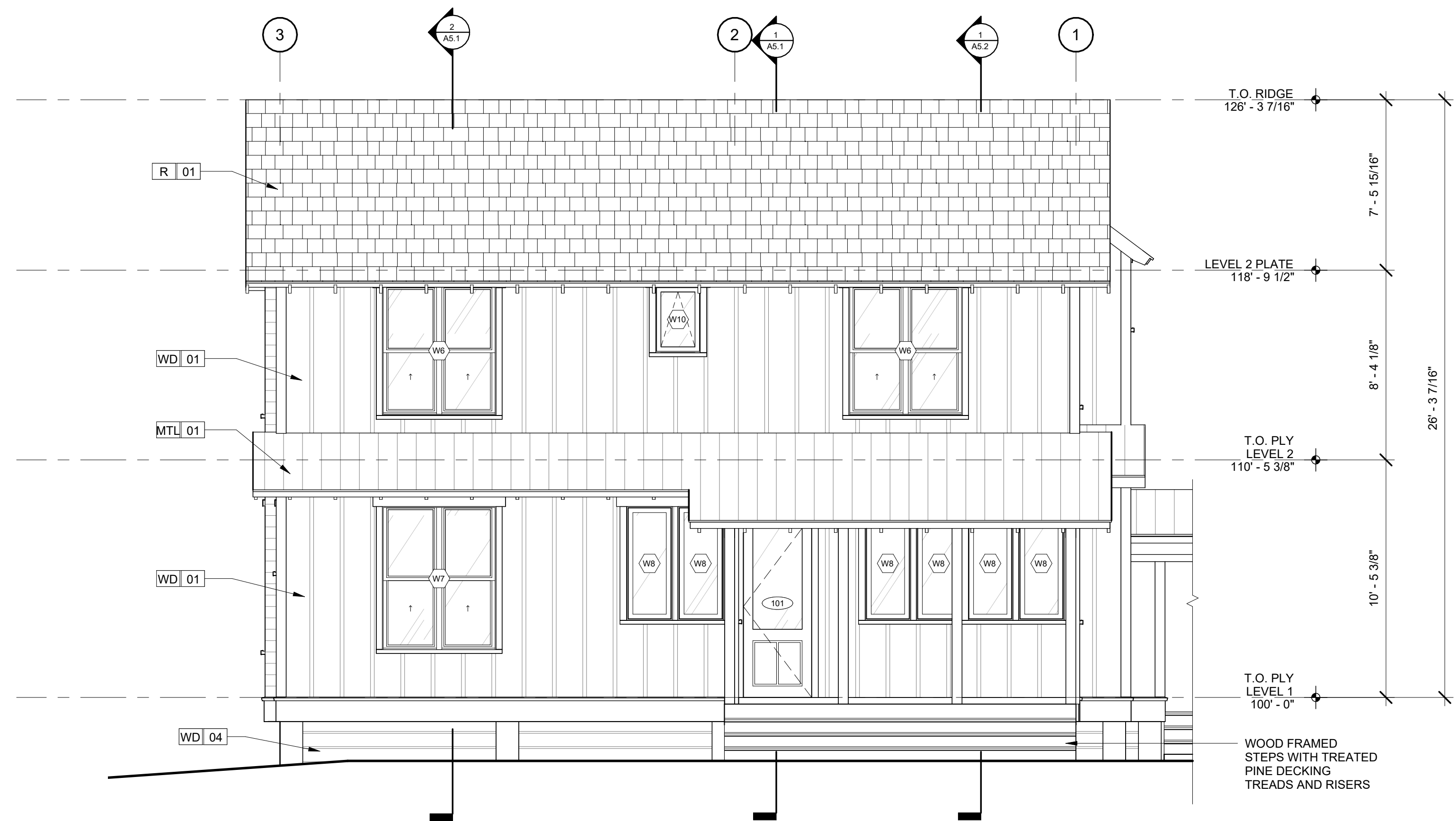
3 NORTH ELEVATION A4.1 SCALE: 1/4" = 1'-0"
