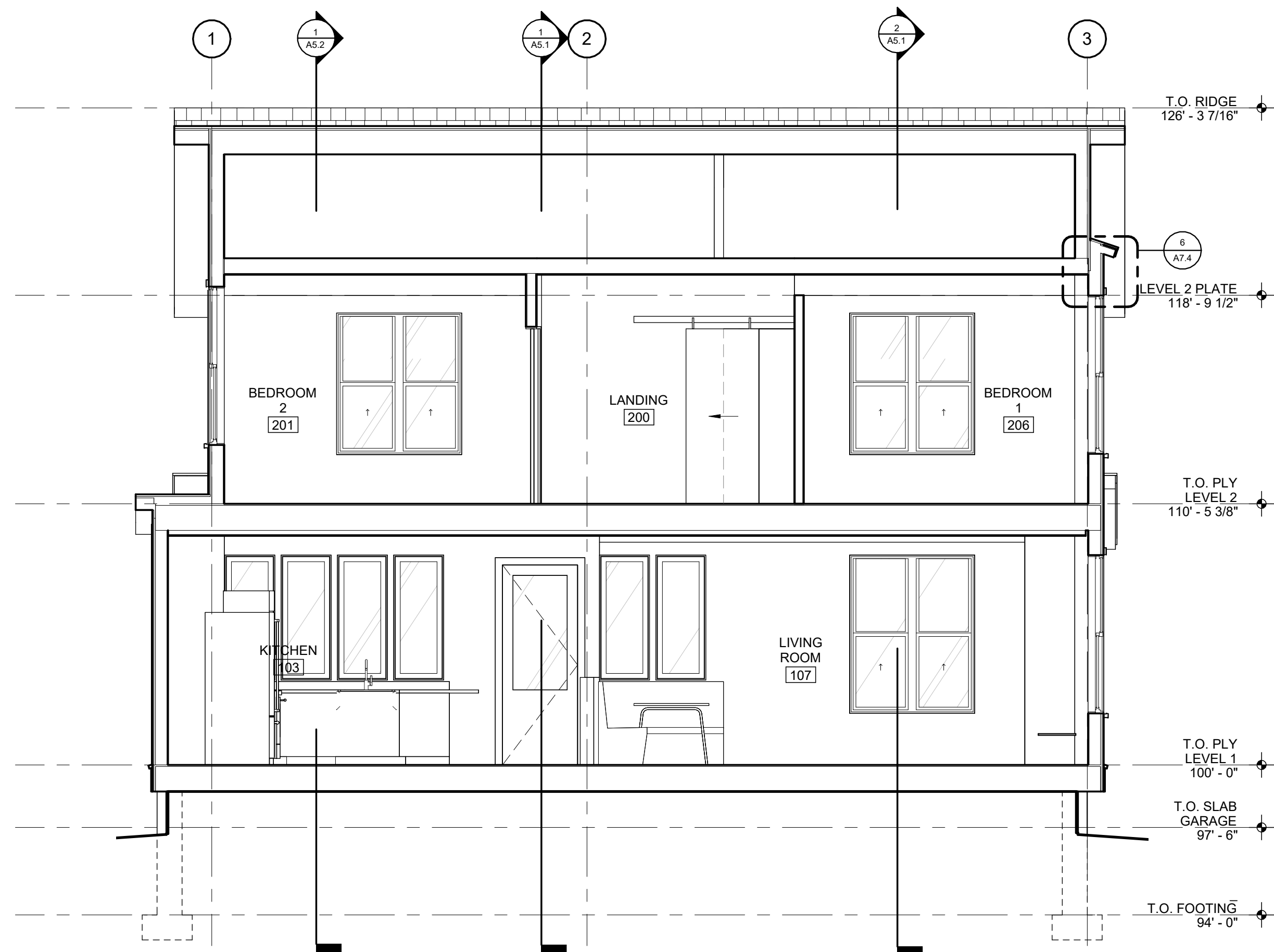
4 BUILDING SECTION A5.1 SCALE: 1/4" = 1'-0"
