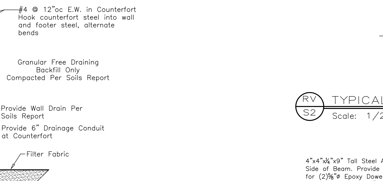
V FOUNDATION DETAIL V S2 Scale: 1/2"=1'-0"
