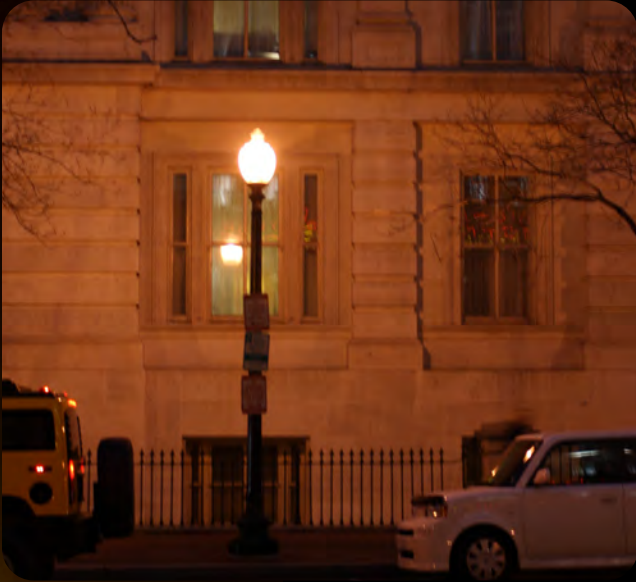
LIGHT TRESPASS When light falls where it is not wanted or needed. Use fully shielded light fixtures whenever possible.
