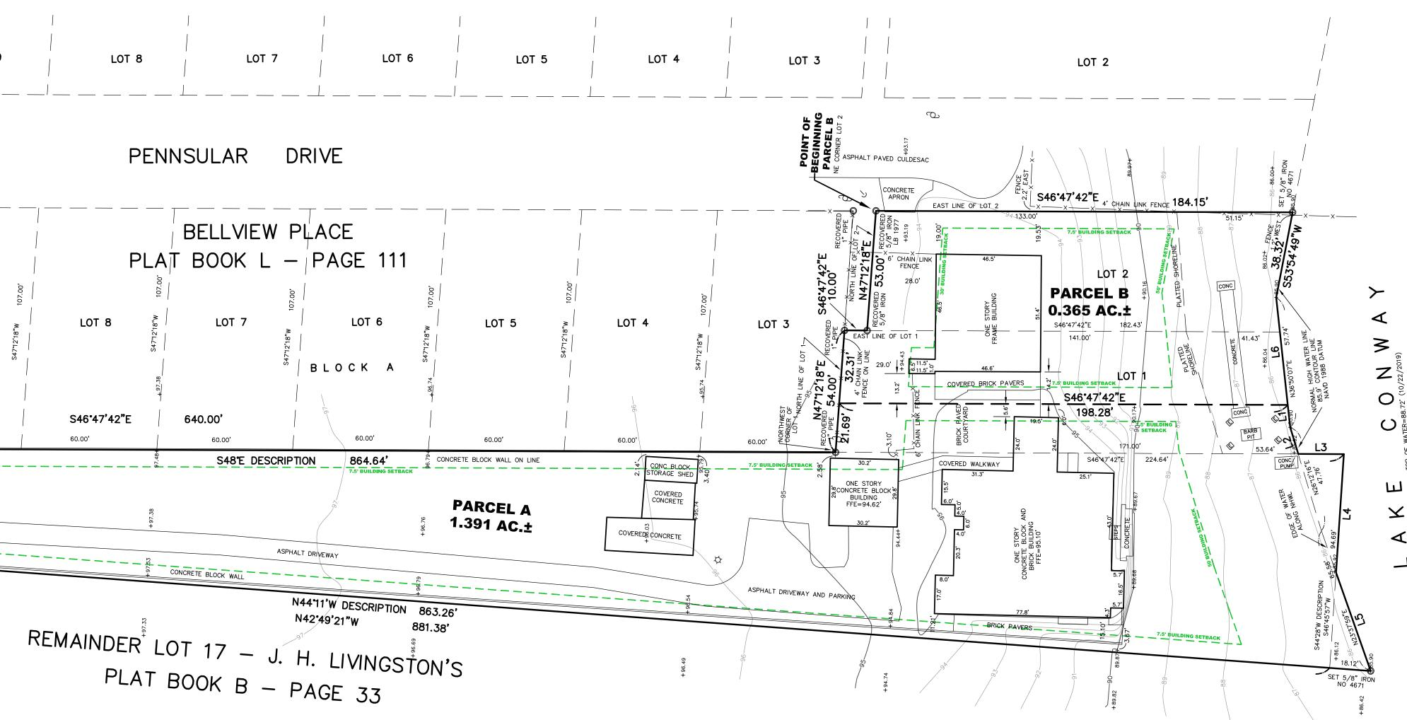
NOTES: - BEARINGS BASED ON THE SOUTH RIGHT OF WAY LINE OF HOFFNER AVENUE AS BEING S47'12'18"W.. - NO UNDERGROUND UTILITIES WERE LOCATED. - ELEVATIONS BASED ON ORANGE COUNTY BENCHMARK NUMBER C1139011. A 2-1/2" BRASS ORANGE COUNTY CONTROL DISK IN CONCRETE CURB MEDIAN AT THE ENTRANCE OF THE HIGHLANDS AT LAKE CONWAY, 2ND MEDIAN IN, 100' NORTHWEST OF CENTERLINE OF HOFFNER AVENUE AT PENINSULAR DRIVE. ELEVATION=94.804', NAVD 1988 DATUM.
