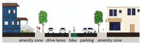
A typical suburban road section should provide adequate space for pedestrians, cyclists, and vehicles with some level of streetscaping.
