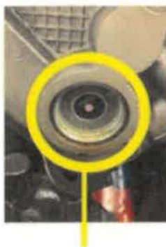
Overheated Pink Sensor 255°F Coolant Temp
