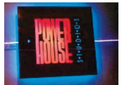
A combination of routed and backed up copy out of a halo illuminated panel
