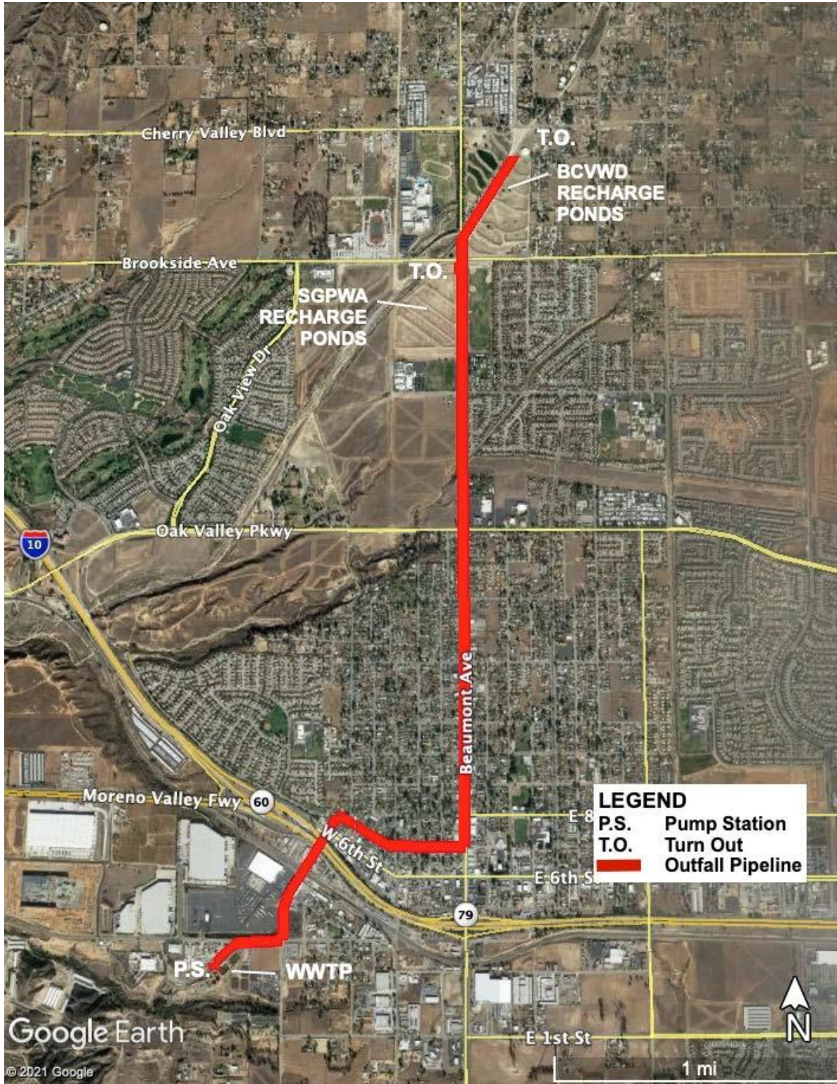
Figure 4-1 Preliminary Outfall from WWTP to Recharge Ponds
