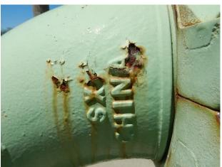
Corrosion typical where coating has flaked
