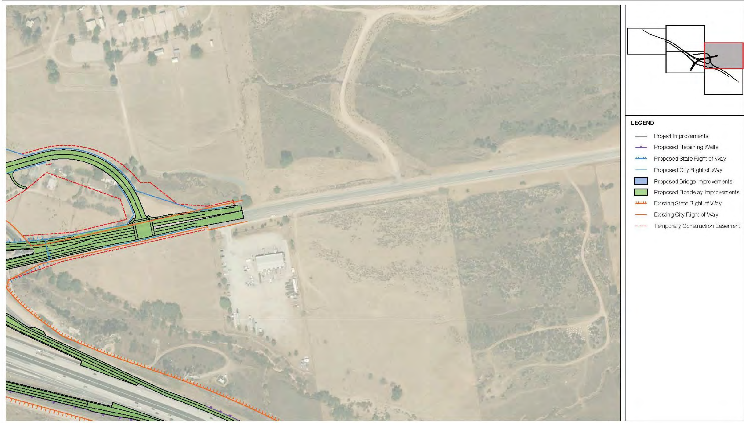
Figure 1-5d: Build Alternative 4 (Partial Cloverleaf)
