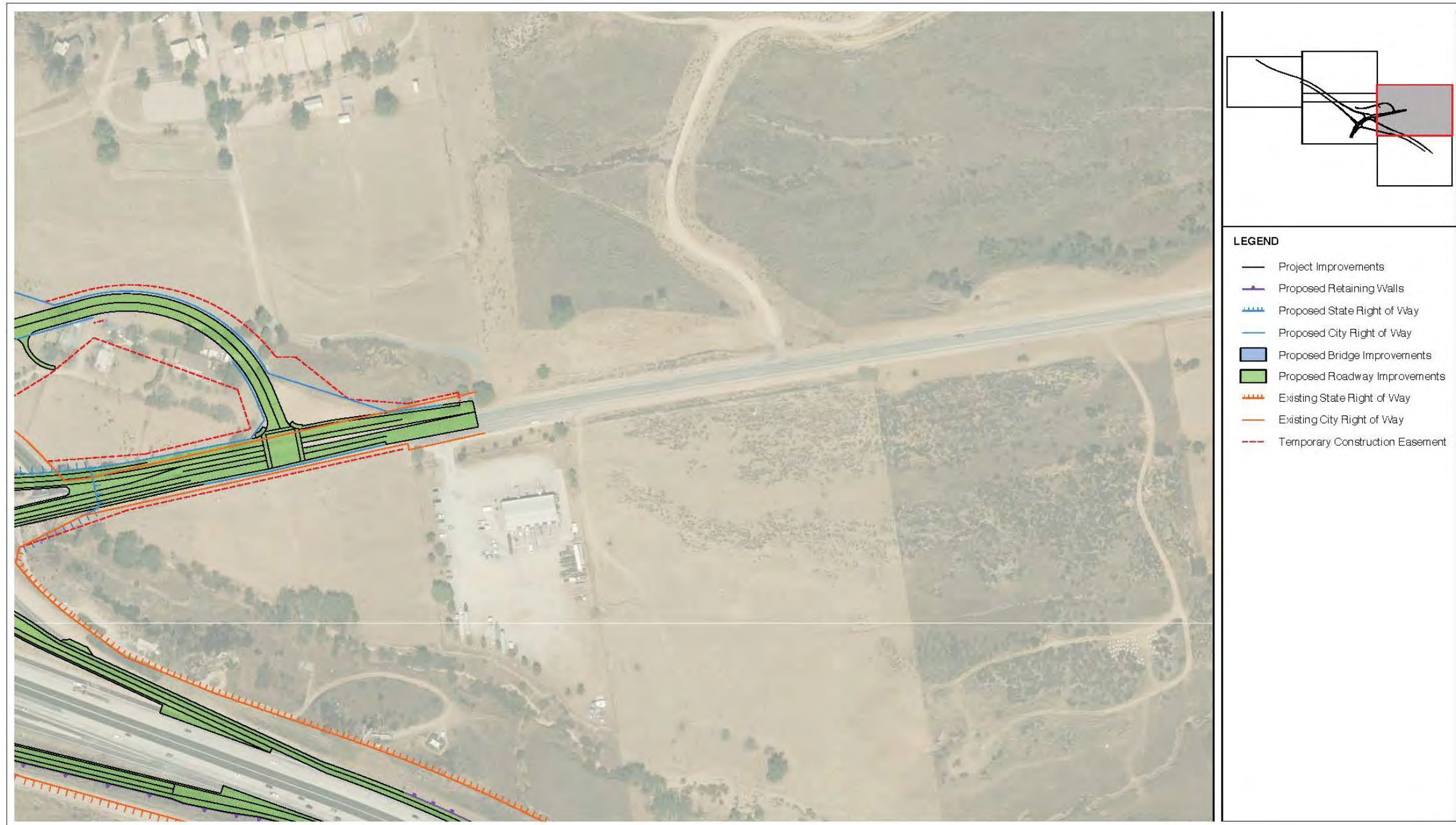
Figure 1-4d: Build Alternative 3 (Diverging Diamond)
